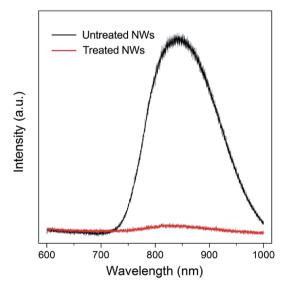
Fig. 3 Photoluminescence (PL) spectra of  $TiO_2$  NW arrays without treatment (black line) and with treatment (red line). The untreated NWs exhibit a strong NIR PL peak centered at about 835 nm, while the PL peak intensity is significantly reduced for the NWs after treatment in  $H_2O_2$ – $NH_3$  (aq) solution for 10 min.
