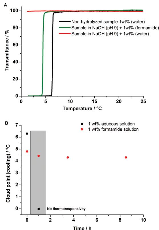
**Fig. 7** (A) Hydrolysis stability of poly(AAm<sub>87</sub>-co-AN<sub>12</sub>) in NaOH (pH 9), with and without sacrificial additives. (B) Stability of the thermoresponsive behavior in aqueous media of poly(AAm<sub>87</sub>-co-AN<sub>12</sub>) at 85 °C depending on time, with and without sacrificial additives.
