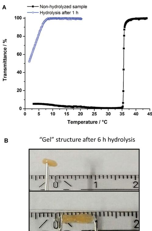
**Fig. 6** (A) Turbidity curves (upon cooling) of poly(AAm<sub>70</sub>-co-AN<sub>16</sub>) before and after hydrolysis in NaOH pH 14 at 40 °C. The polymers were dissolved in HCl solutions (pH 3, 1 wt%). (B) Interpolymer complex “gel” in pH 3 (hydrolyzed sample over 6 h in NaOH pH 14 at 40 °C).
