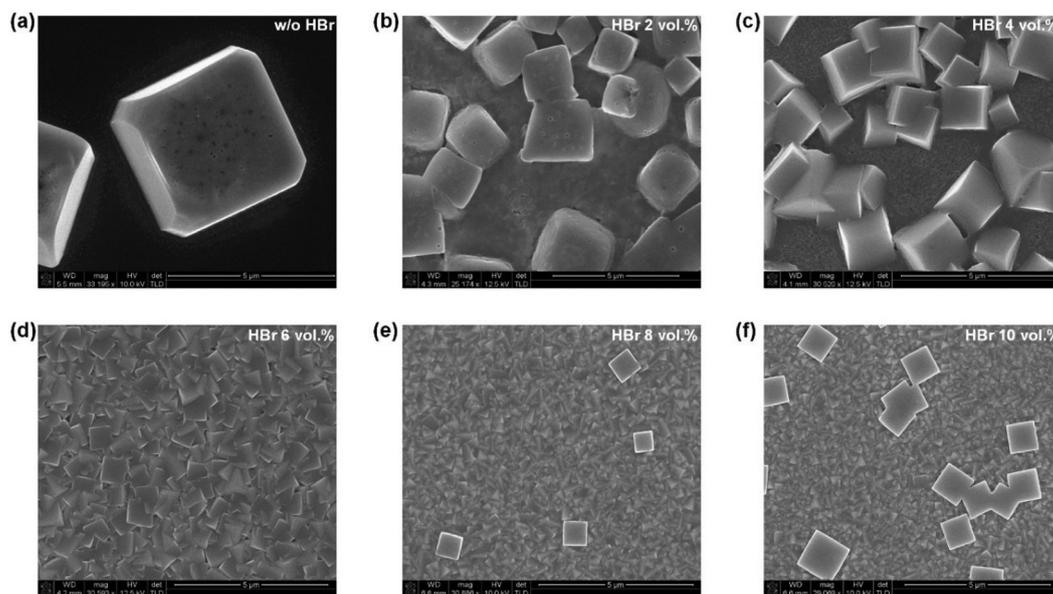
Fig. 2 SEM images of the top surfaces of the MAPbBr<sub>3</sub> layers deposited using 0–10 vol% of HBr in the DMF/HBr cosolvent on PEDOT:PSS-coated ITO/glass substrates.
