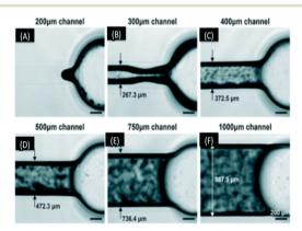
Fig. 11 (A-F) Micrographs of 500 μm tall channels built in a range of widths. The actual width of each channels showed deviation of almost 30  $\mu$ m from design. The 300  $\mu$ m wide channel could only be partially cleared of resin, while the smaller channels did not clear at all and larger channels were fully cleared. 60 (Copyright 2015 RSC).
