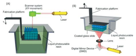
Fig. 7 Two SLA printing configurations. (A) Laser-scanning SL with the free surface/bath configuration. (B) DLP SLA with the constrained-surface/"bat" configuration. (Copyright 2015 Elsevier).
