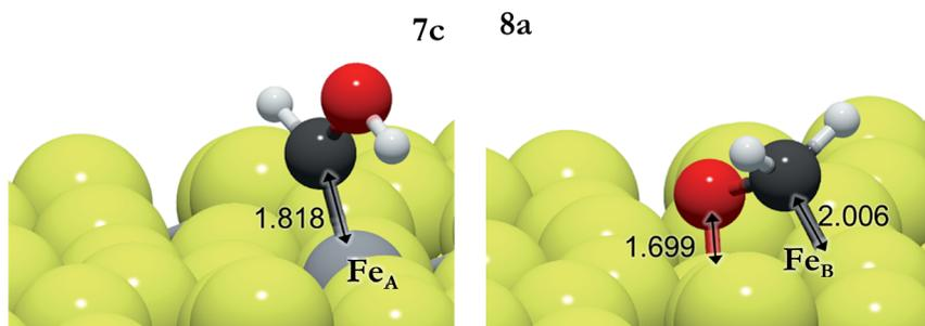
**Fig. 5** Schematic representation of HCOH (from **7c**) on Fe<sub>A</sub> (left) and H<sub>2</sub>CO (from **8a**) on Fe<sub>B</sub> (right). The light grey and yellow balls represent Fe and S, respectively, and the red and dark grey balls represent O and C, respectively.
