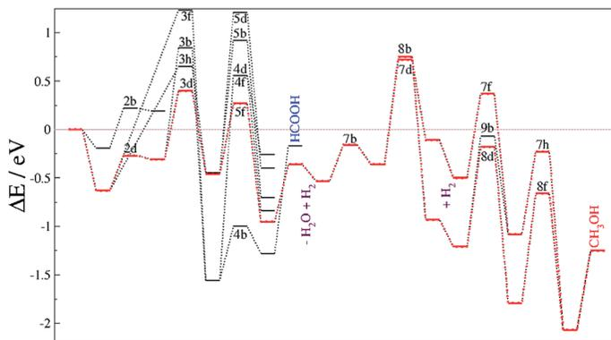
Fig. 7 Reaction energy profiles for the  $\text{CO}_2$  hydrogenation process taking place on  $\text{Fe}_B$ . The blue line highlights the formate pathway. The labels corresponding to elementary steps are placed at the transition state. Processes such as water molecule release ( $-\text{H}_2\text{O}$ ) and surface hydrogenation ( $+\text{H}_2$ ) are also included. The horizontal brown line indicates the energy reference of the naked surface and isolated molecules.
