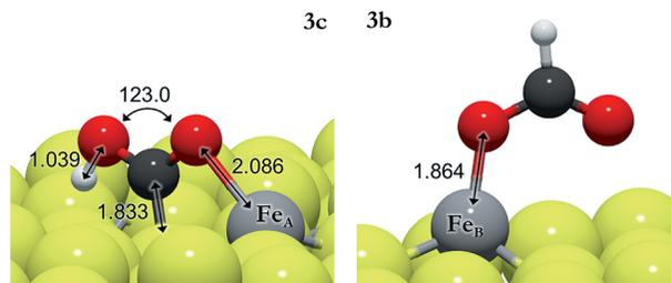
Fig. 2 Schematic representation of hydrocarboxyl (from **3c**) on  $\text{Fe}_A$  (left) and formate (from **3b**) on  $\text{Fe}_B$  (right). The light grey and yellow balls represent Fe and S, respectively, and the red and dark grey balls represent O and C, respectively.
