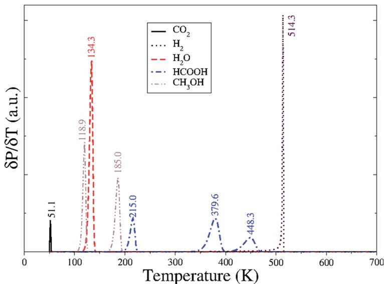
Fig. 8 Temperature programmed desorption of the molecules involved in the reduction mechanism of  $\text{CO}_2$  on  $\text{Fe}_3\text{S}_4(111)$ . The temperature range considered is from 50 to 700 K, evaluated every 2 K each 2 s, leading to a heating rate of  $1 \text{ K s}^{-1}$ .
