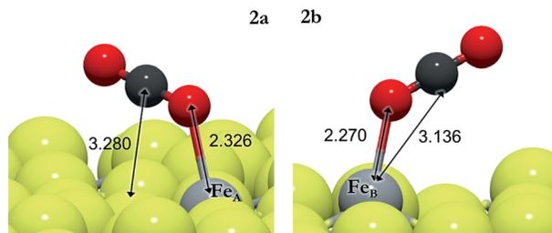
Fig. 1 Schematic representation of non-activated CO<sub>2</sub> on Fe<sub>A</sub> (left) and on Fe<sub>B</sub> (right). The light grey and yellow balls represent Fe and S, respectively, and the red and dark grey balls represent O and C, respectively.
