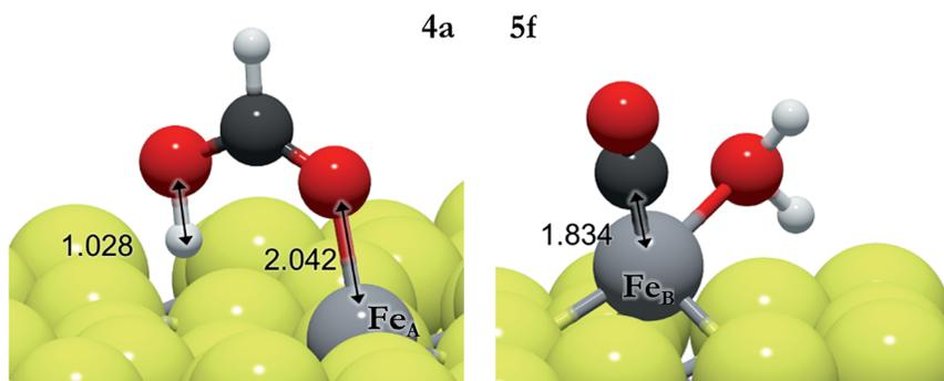
**Fig. 3** Schematic representation of HCOO<sup>1</sup>H (from **4a**) on Fe<sub>A</sub> (left) and CO + H<sub>2</sub>O (from **5f**) on Fe<sub>B</sub> (right). The light grey and yellow balls represent Fe and S, respectively, and the red and dark grey balls represent O and C, respectively.
