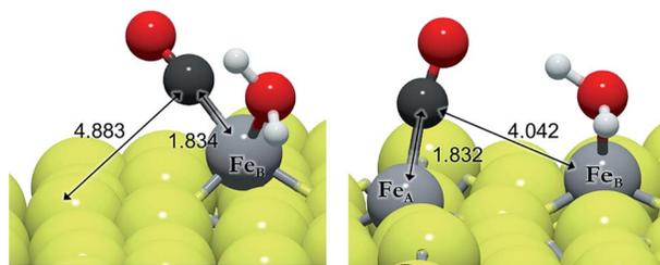
Fig. 4 Schematic representation of CO migration from  $\text{Fe}_B$  (left) to  $\text{Fe}_A$  (right) according to the process **6a**. The light grey and yellow balls represent Fe and S, respectively, and the red and dark grey balls represent O and C, respectively.
