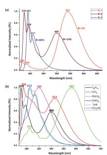
Fig. 5 (a) Normalized PL of **M-1** (20  $\mu$ M), **M-2** and **M-3** (2  $\mu$ M) in C<sub>6</sub>H<sub>12</sub>; (b) normalized PL of **M-2** (2  $\mu$ M) in different solvents, both were excited at 350 nm
