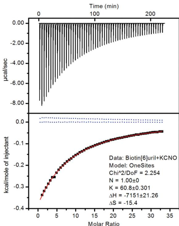
Fig. 3 ITC of Biotin[6]juril with KCNO in 100 mM phosphate buffer at pH 7.5 at 30 °C. Black: observed data, Red: fitted data, Blue: dilution contribution.  $K$  ( $M^{-1}$ ),  $\Delta H$  ( $\text{cal mol}^{-1}$ ) or  $\Delta S$  ( $\text{cal mol}^{-1} \text{deg}^{-1}$ ).
