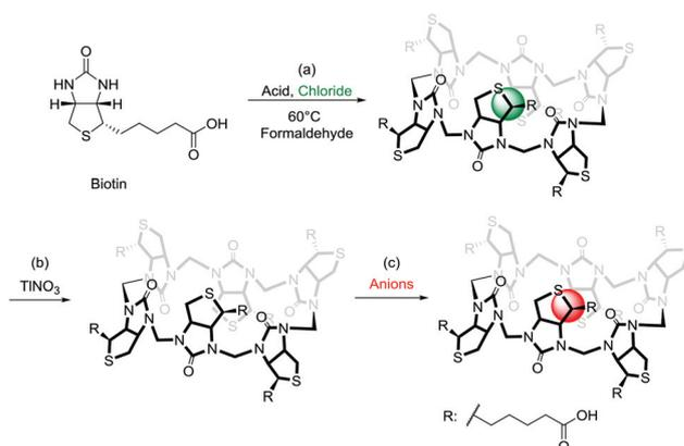
**Fig. 1** (a) Synthetic route to Biotin[6]uril (with chloride or bromide encapsulated, green), (b) synthesis of anion-free Biotin[6]uril and (c) the reincorporation of other anions (red) studied in this work.
