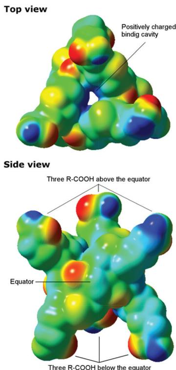
**Fig. 4** Electrostatic surface potential of Biotin[6]juril at the CAM-B3LYP/6-31G(d) level of theory. Top view: showing the central binding cavity with a positive electrostatic potential. Side view: showing that the macrocycle has three carboxylic acids pointing in either direction of the equator of the macrocycle defined as the area surrounding the binding cavity. Red:  $-31 \text{ kcal mol}^{-1}$  blue:  $+31 \text{ kcal mol}^{-1}$ .
