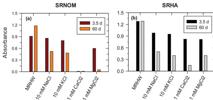
Fig. 12 Plot demonstrating the stability of SRNOM- and SRHA-formed Ag nanoparticles in 1 h at 410 nm in chloride solutions by monitoring the absorbance of SPR peaks. ( $[Ag^+] = 1 \times 10^{-3}$  M,  $[SRNOM] = [SRHA] = 15$  mg L<sup>-1</sup> in moderately hard reconstituted water (MRHW) at pH 8.0 and 90 °C). (SRNOM – Suwannee river natural organic matter; SRHA – Suwannee river humic acid). (Adapted with permission from ref. 25, copyright Elsevier Inc.)
