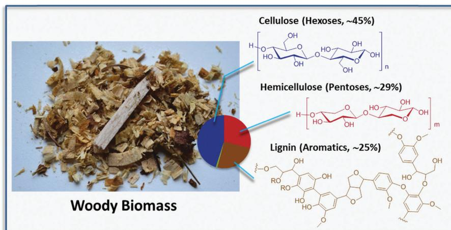
Fig. 1 Schematic representation of woody biomass composition.
