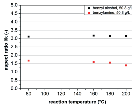
Fig. 10 Influence of the reaction temperature on the aspect ratio of the AZO nanocrystals prepared in BnOH and BnNH 2 .
