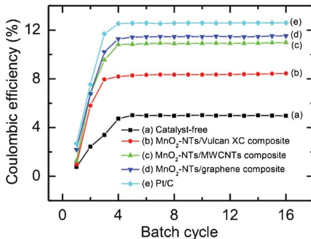
**Fig. 7** Coulombic efficiency (%) of sMFC as a function of batch cycle with (a) catalyst-free, (b)  $\text{MnO}_2$ -NTs/Vulcan XC, (c)  $\text{MnO}_2$ -NTs/MWCNTs, (d)  $\text{MnO}_2$ -NTs/graphene, and (e) Pt/C composite cathodes. Each batch cycle was  $36 \text{ h} (\pm 2 \text{ h})$ .
