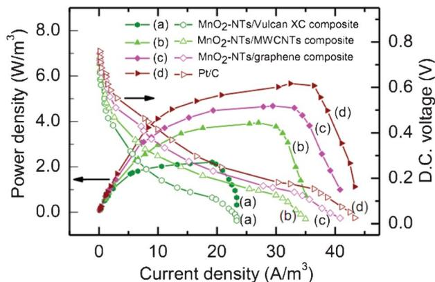
**Fig. 5** Polarization plots for sMFC (power density and DC voltage as a function of current density) with different air cathodes (a) MnO<sub>2</sub>-NTs/Vulcan XC (b) MnO<sub>2</sub>-NTs/MWCNTs, (c) MnO<sub>2</sub>-NTs/graphene, and (d) Pt/C composites. The power density and voltage data points are presented as solid and open symbols, respectively. A fixed quantity of catalyst (0.3 gm/cm<sup>2</sup> MnO<sub>2</sub>-NTs or Pt) was loaded onto different carbon supports for comparison.
