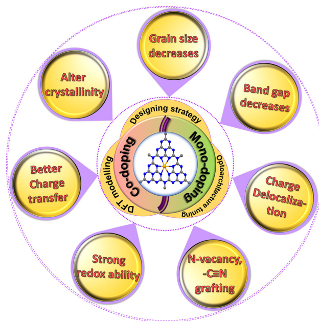
Fig. 2 Schematic illustration of the effect of alkali-doping in the g\text{-C}_3\text{N}_4 matrix.
