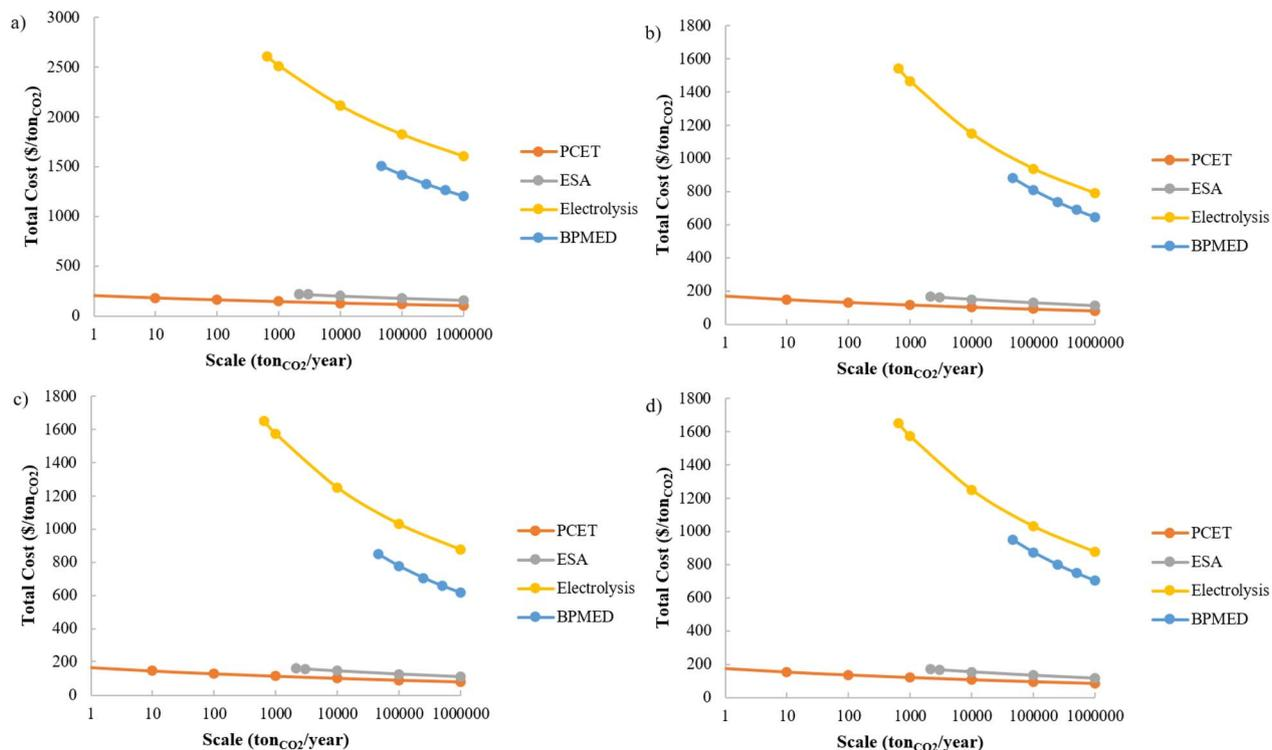
Fig. 9 Total costs of e-DAC technologies located in Europe for the year 2023 when (a) nuclear, (b) solar, (c) on-shore wind, and (d) off-shore wind energies are used.
