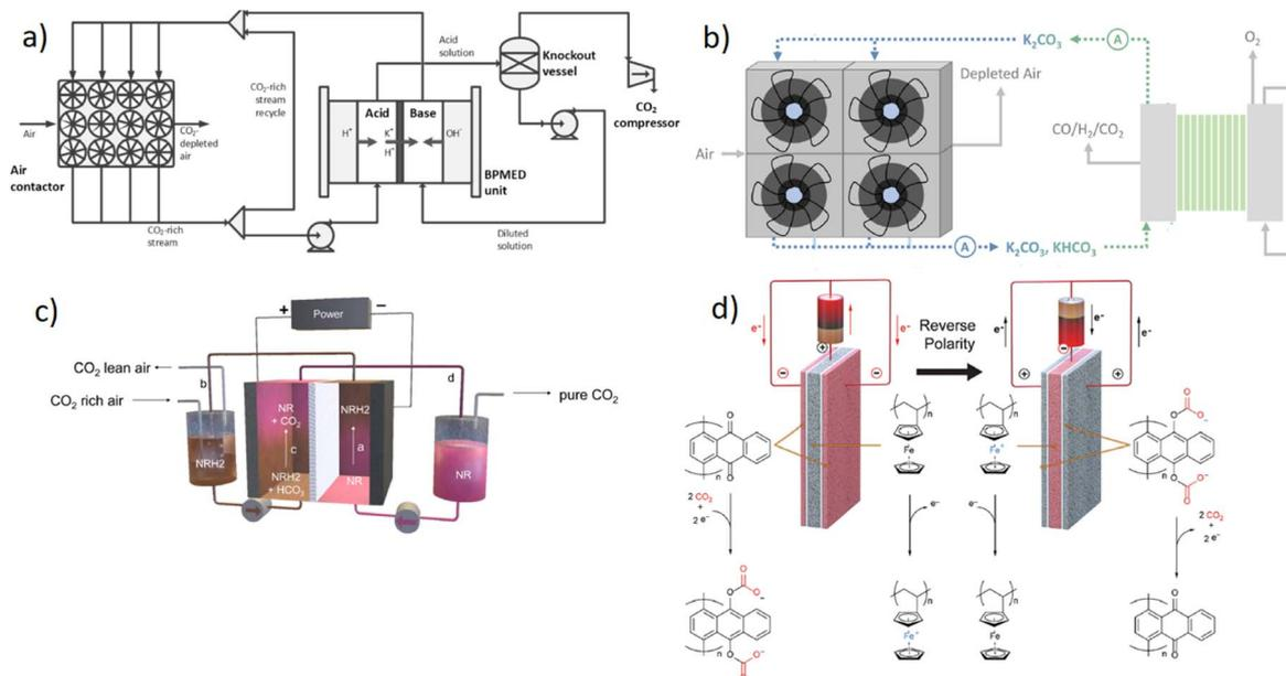
Fig. 2 Scheme of the operating principle of e-DAC technologies: (a) BPMED, (b) electrolysis, (c) PCET, and (d) ESA.<sup>20,29,34,43</sup>
