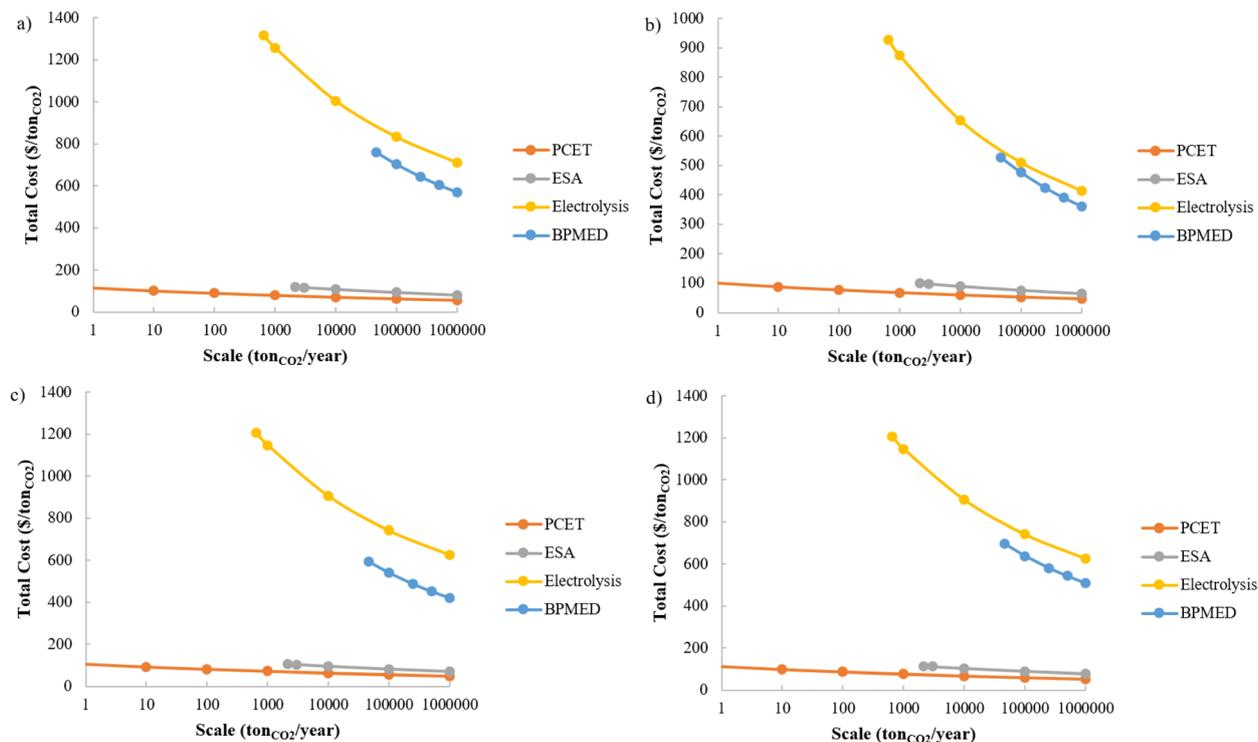
Fig. 7 Total costs of e-DAC technologies located in China for the year 2030 when (a) nuclear, (b) solar, (c) on-shore wind, and (d) off-shore wind energies are used.
