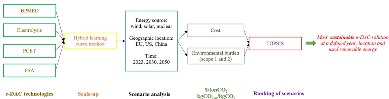
Fig. 1 Workflow diagram of the used computational methodology.
