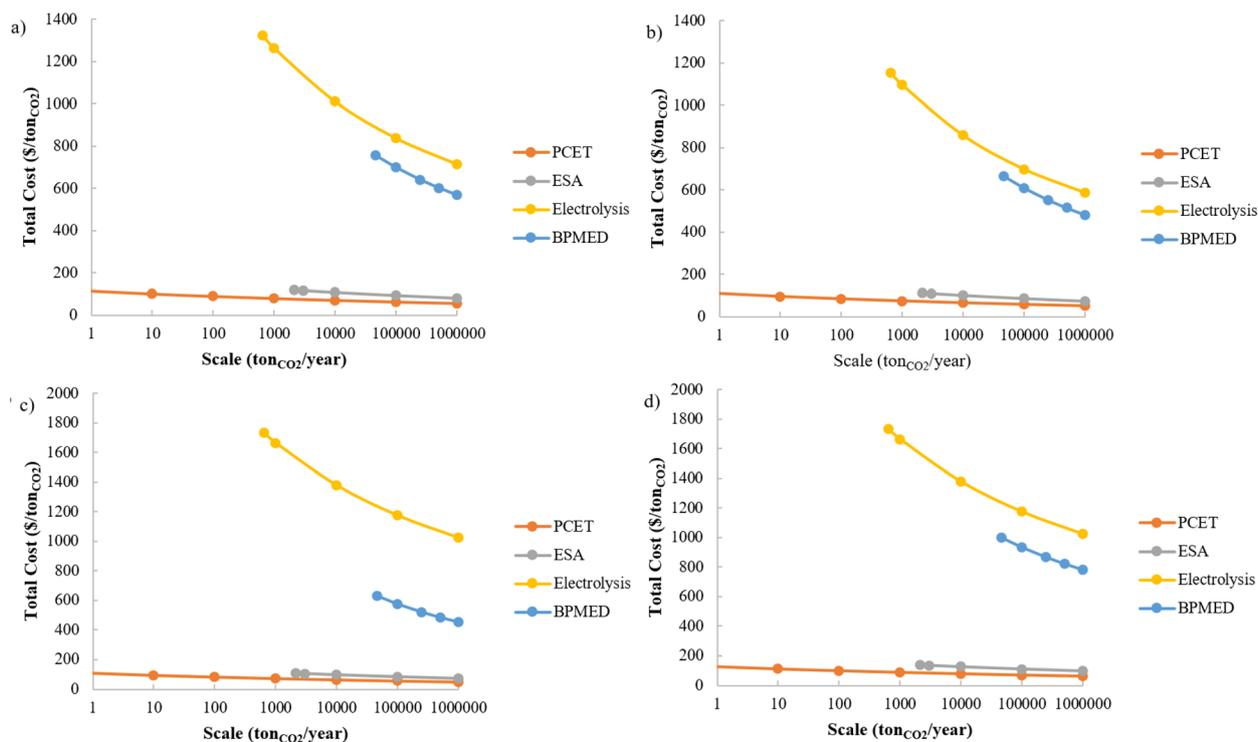
Fig. 6 Total costs of e-DAC technologies located in China for the year 2023 when (a) nuclear, (b) solar, (c) on-shore wind, and (d) off-shore wind energies are used.
