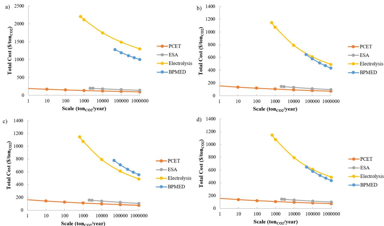
Fig. 11 Total costs of e-DAC technologies located in Europe for the year 2050 when (a) nuclear, (b) solar, (c) on-shore wind, and (d) off-shore wind energies are used.
