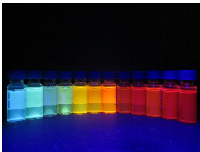
Fig. 3 Photograph of continuously synthesised \text{Zn}_3\text{N}_2 samples at UV-light (left) and their corresponding coordinates in the CIE colour map (right). A broad fluorescence wavelength spectrum can be manufactured in a continuous synthesis manner, namely 506 to 710 nm (left). \text{Zn}_3\text{N}_2 QDs inherently offer high colour purity as their emission spectra correspond to CIE coordinates at the edge of the respective colour gamut (right). Here, the dotted triangle spans the standardised Adobe RGB (1998) colour space, thus \text{Zn}_3\text{N}_2 QDs exceed this region.
