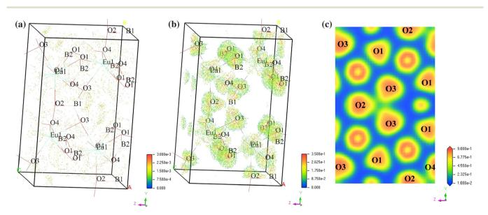
Fig. 5 The unoccupied (a) and occupied (b) SHG densities of RNEBO. (c) The electron localization function (ELF) map of RNEBO.
