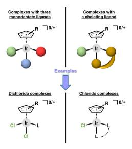
Fig. 3 Two basic structural types of half-sandwich iridium(III) cyclopentadienyl complexes (Ir-Cpx).
