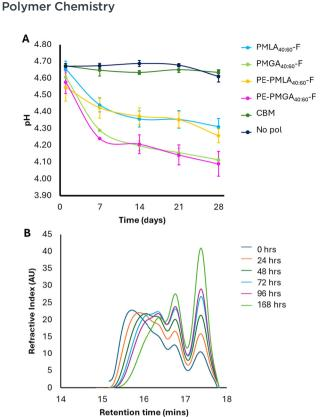
Fig. 6 Polymer degradation. (A) pH changes in shampoo formulations as a function of time. (B) Gel permeation chromatograms of PMLA $_{40:60}$ -F when incubated in pH 4 buffer as a function of time.
