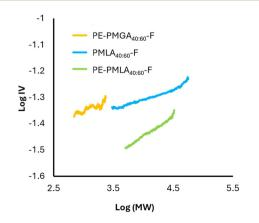
Fig. 4 Mark-Houwink plot of aqueous soluble polyesters. IV = intrinsic viscosity; MW = molecular weight.
