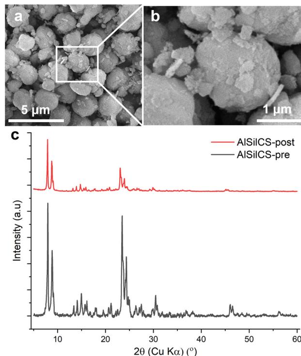
Fig. 7 Characterization of post-reaction catalyst. (a) SEM image of Al-Sil-CS post reaction (scale =  $5 \mu\text{m}$ ), (b) SEM image of Al-Sil-CS post reaction (scale =  $1 \mu\text{m}$ ), (c) an overlay of the X-ray diffractograms for the Al-Sil-CS catalyst, showing the structure pre and post reaction.
