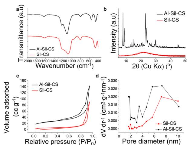
**Fig. 5** Structural comparison of Sil-CS (red) and Al-Sil-CS (black). (a) FTIR spectra showing Si–O–Si vibrations and 5MR band in Al-Sil-CS, (b) XRD diffractograms indicating amorphous silica in Sil-CS and crystalline MFI-type framework in Al-Sil-CS, (c)  $\text{N}_2$  adsorption–desorption isotherms showing increased surface area of Al-Sil-CS compared to Sil-CS, and (d) BJH pore size distribution of Sil-CS and Al-Sil-CS.
