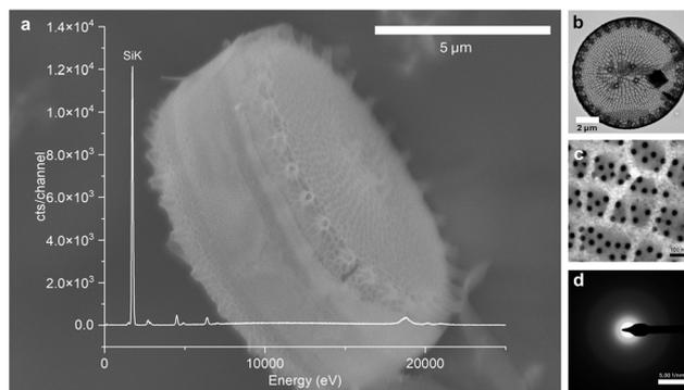
**Fig. 2** Characteristics of *C. striata* TBI biosilica (Sil-CS). (a) SEM image of Sil-CS (scale = 5  $\mu\text{m}$ ) with overlaid XRF spectrum showing a dominant Si K- $\alpha$  emission, (b) TEM image of Sil-CS (scale = 2  $\mu\text{m}$ ), (c) TEM image of interlayer hierarchical pores on Sil-CS surface (scale = 100 nm), and (d) selected area electron diffraction (SAED) pattern of Sil-CS (scale = 100 nm).
