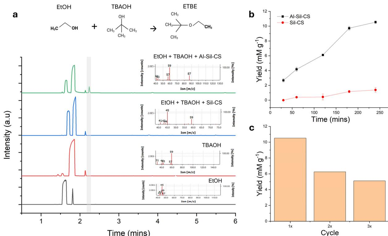
**Fig. 6** Catalytic performance of Al-Sil-CS in ETBE synthesis. (a) GC-MS chromatogram highlighting ETBE peak (grey) and its corresponding mass fragments, (b) comparison of ETBE production yield using Al-Sil-CS (black) and Sil-CS (red), and (c) catalytic reusability of Al-Sil-CS over multiple cycles.
