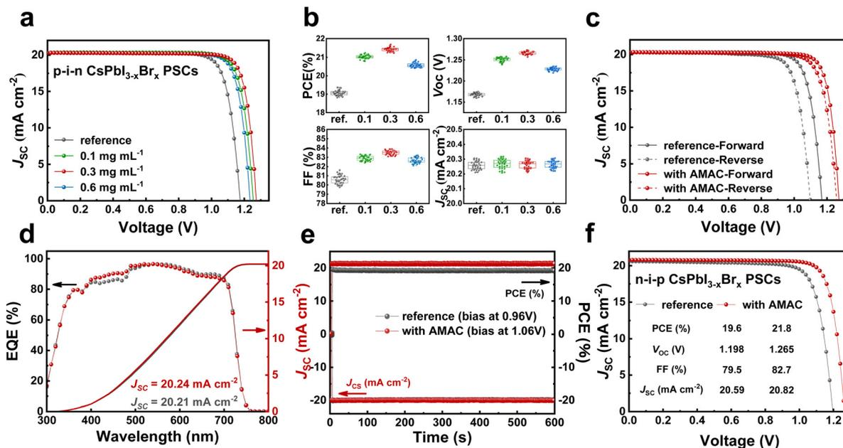
Fig. 4 (a)  $J$ - $V$  characterization of p-i-n CsPbI<sub>3-x</sub>Br<sub>x</sub> PSCs incorporated with different amounts of AMAC under 100 mW cm<sup>-2</sup> illumination (the active area is 0.09 cm<sup>2</sup>). (b) Statistical box charts of PV parameters. (c) Hysteresis with and without AMAC-incorporated PSCs. (d) EQE and integrated  $J_{SC}$ . (e) SPO at MPP tracking. (f)  $J$ - $V$  characterization of n-i-p CsPbI<sub>3-x</sub>Br<sub>x</sub> PSCs with and without AMAC incorporation.
