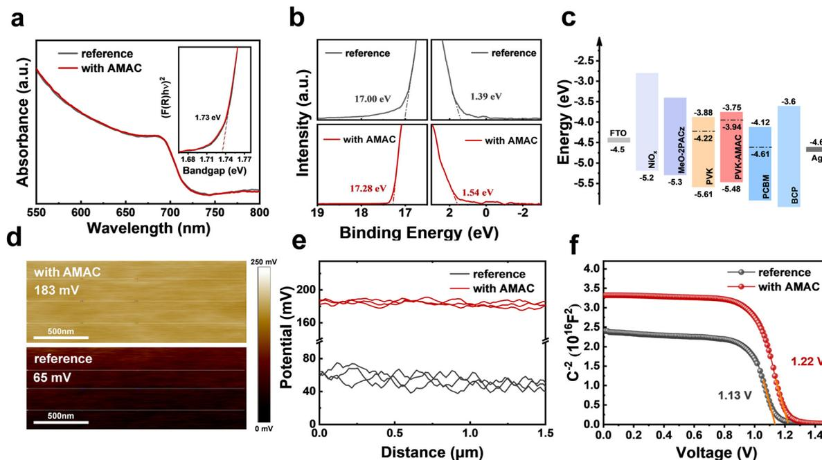
Fig. 6 (a) UV-vis spectra of films with and without AMAC incorporation (inset: Tauc plot). (b) UPS patterns of perovskite films with and without AMAC incorporation. (c) Energy diagram (vs. vacuum). (d) and (e) KPFM images and corresponding surface potential. (f)  $C-V$  characteristic plots of devices.
