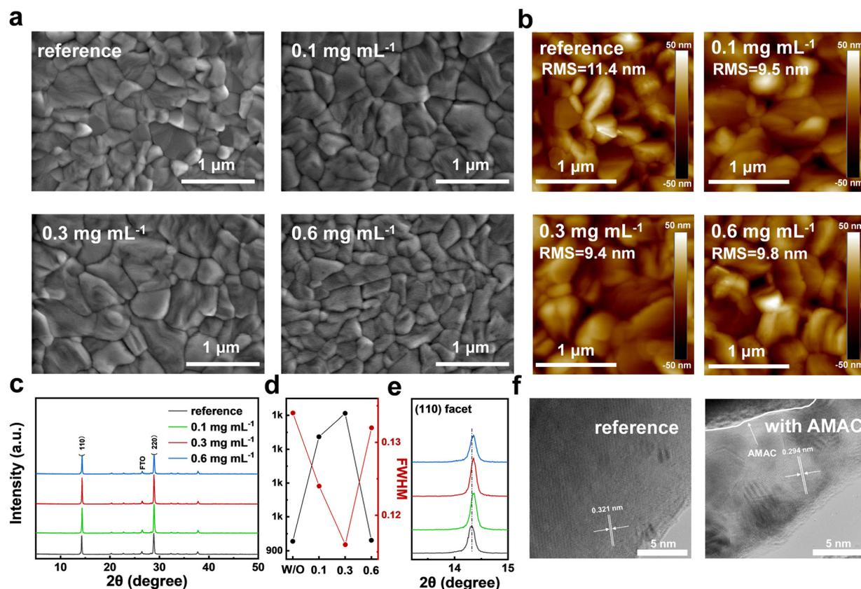
Fig. 2 (a) Top-view SEM images with different concentrations of AMAC incorporation. (b) AFM images of perovskite films with different concentrations of AMAC incorporation. (c) XRD patterns of inorganic perovskite films with different concentrations of AMAC incorporation. (d) Peak intensity and FWHM derived from XRD patterns. (e) XRD patterns of the perovskite (110) facet. (f) TEM images of inorganic perovskite films.
