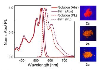
Fig. 7 Absorption (Abs, solid lines) and emission (PL, dashed lines) of compound 3a in dichloromethane (red) and in neat thin film (dark red). The clear vibronic progression is retained for both absorption and emission spectra of the neat film (left). Photographs of OAPPDOs 2a, 2e and 3a as powders under UV-illumination ( $\lambda_{exc}$  = 365 nm, right).
