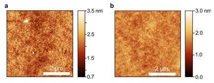
Fig. 4 Atomic force microscopy images of a neat film of (a) compound 2d and (b) compound 3a. The scale bar is 2 µm.
