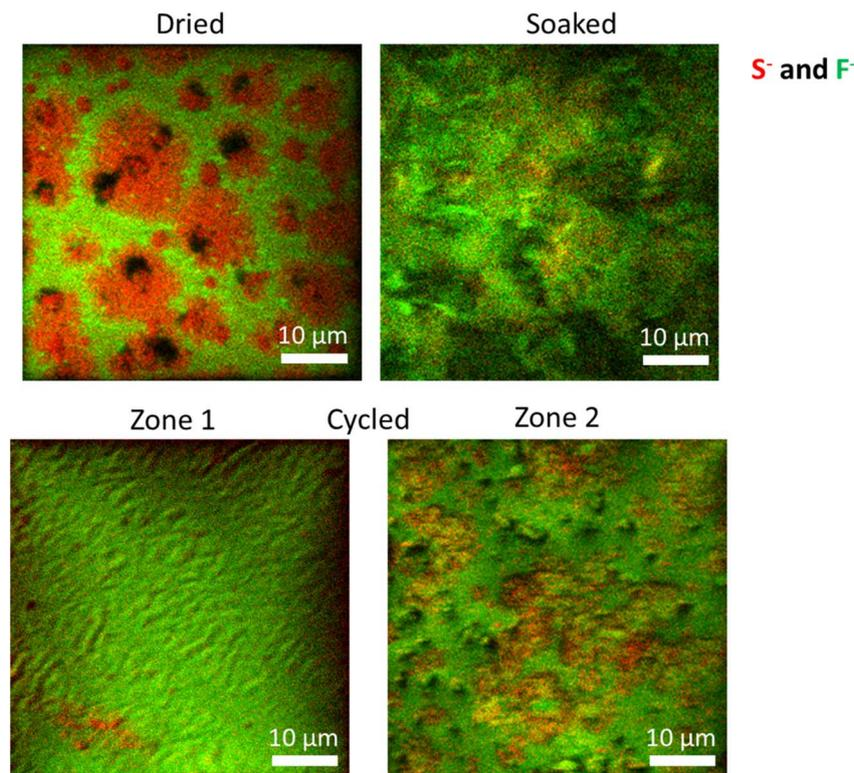
Fig. 6 ToF-SIMS combined mappings of  $S^-$  (red) and  $F^-$  (green) ionic fragments on the surface of the NaSTFSI-co-PET-MP/4A membrane (dried), incorporating EC : DMC : FEC molecular transporters (soaked) and after cycling for 5 cycles in a Na|Na symmetric cell under  $10 \mu A cm^{-2}$  (cycled).
