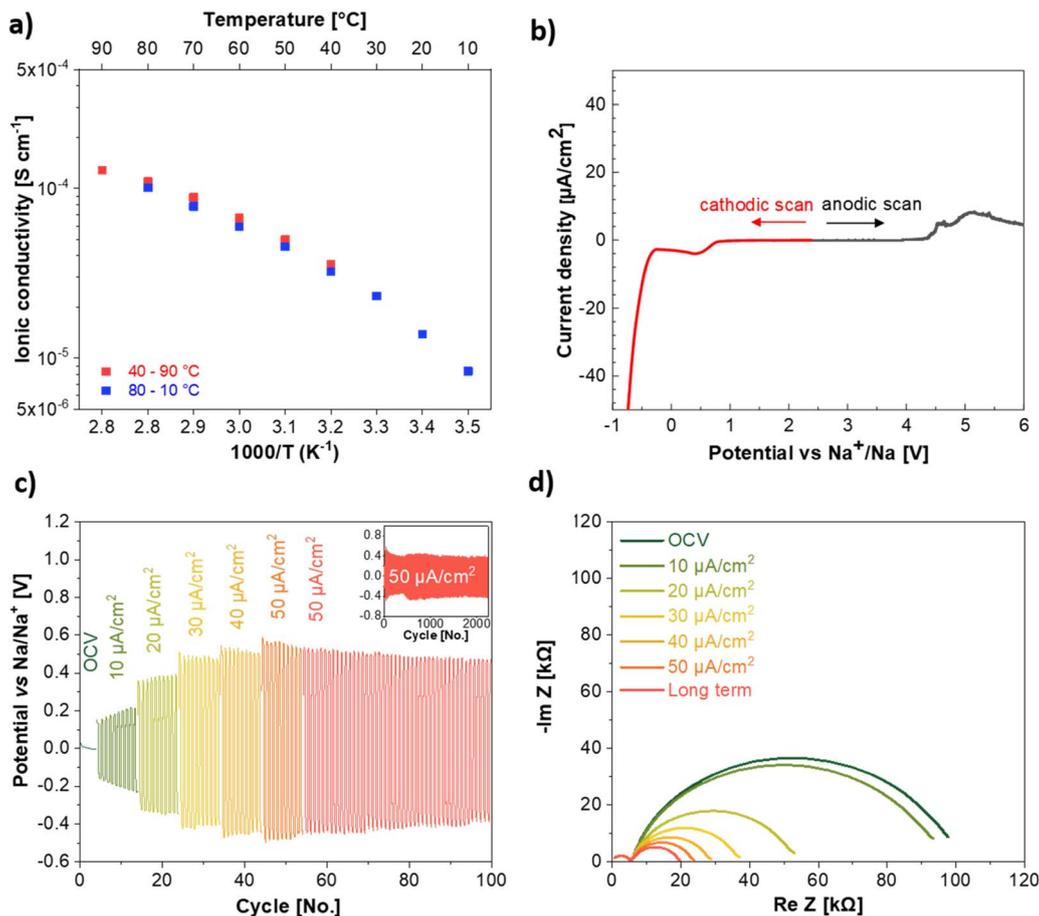
Fig. 4 Electrochemical characterization of NaSTFSI-co-PET-MP/4A electrolyte: (a) ionic conductivity in the temperature range of 10–90 °C; (b) anodic and cathodic scan in Na|Al cells; (c) Na stripping/plating test over 2000 h at different current densities in Na|Na symmetric cells, and (d) the corresponding Nyquist plot after cycling for 10 cycles at each current density. Additionally, the EIS was measured after 100 cycles at 50 μA cm<sup>-2</sup> (red line). All tests were performed at 40 °C.
