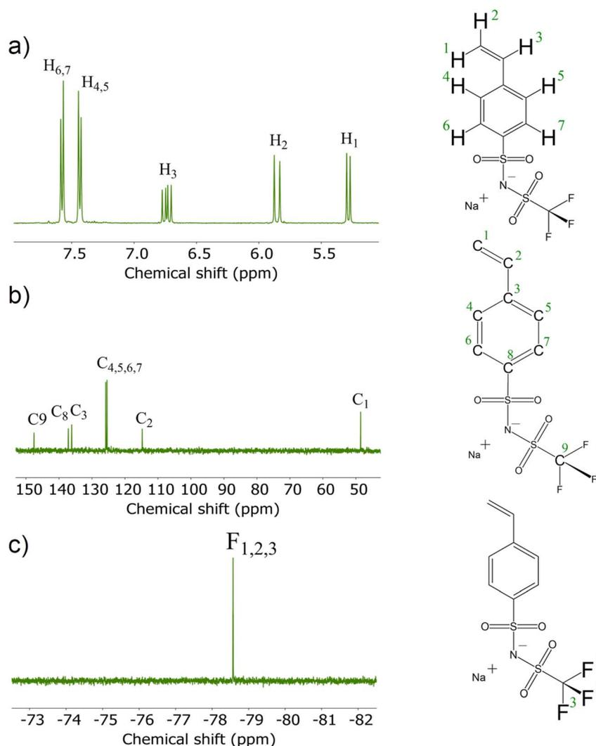
Fig. 1 (a)  $^1\text{H}$ , (b)  $^{13}\text{C}$ , and (c)  $^{19}\text{F}$ -NMR spectra and structure of NaSTFSI sodium salt monomer.
