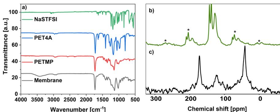
Fig. 2 (a) FT-IR spectra of NaSTFSI, PET4A, PETMP, and NaSTFSI-co-PET-MP/4A membrane.  $^1\text{H} \rightarrow ^{13}\text{C}$  CPMAS NMR spectrum of (b) NaSTFSI and (c) NaSTFSI-co-PET-MP/4A electrolyte, recorded at 10 kHz and 14.1 T. Note: Signals marked with asterisks (\*) are spinning side-bands.
