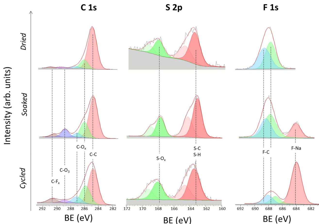
Fig. 5 *Ex situ* C 1s, S 2p, and F 1s XPS spectra of the surface of the NaSTFSI-co-PET-MP/4A membrane (dried), incorporating EC : DMC : FEC molecular transporters (soaked) and after cycling for 5 cycles in a Na|Na symmetric cell under  $10 \mu\text{A cm}^{-2}$  (cycled).
