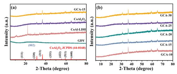
Fig. 2 (a) XRD patterns of GDY, precursor CoAl-LDHs, annealed CoAl<sub>2</sub>O<sub>4</sub> and GCA-15; (b) GCA-X samples.
