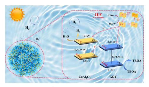
The charge transfer mechanism over the GDY/CoAl<sub>2</sub>O<sub>4</sub> S-scheme heterojunction.
