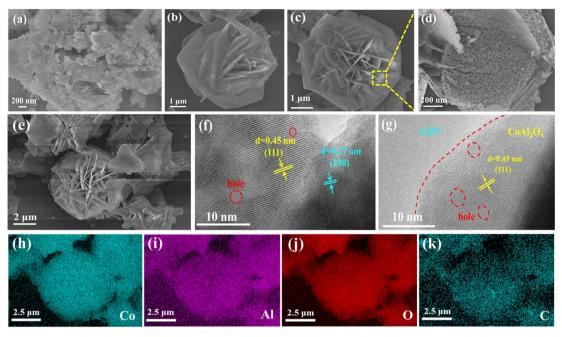
Fig. 4 SEM images of (a) GDY, (b) CoAl-LDHs, (c and d) CoAl<sub>2</sub>O<sub>4</sub> and (e) GCA-15; HRTEM images of (f) CoAl<sub>2</sub>O<sub>4</sub> and (g) GCA-15; elemental mappings (h-k) of the area in (e) for GCA-15.
