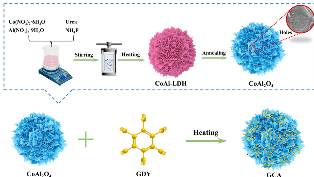
Fig. 1 Schematic of the fabrication process for \text{CoAl}_2\text{O}_4 nanoflowers and the 2D/3D GDY/ \text{CoAl}_2\text{O}_4 heterojunction.
