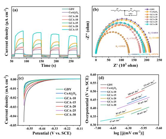
Fig. 12 (a) Transient photocurrent responses for GDY,  $CoAl_2O_4$  and GCA-X; (b) EIS of GDY,  $CoAl_2O_4$  and GCA-X; (c) LSV curves of GDY,  $CoAl_2O_4$  and GCA-X; (c) LSV curves of GDY,  $CoAl_2O_4$  and CCA-X; (c) LSV curves of CCA-X; (c) LSV curves of CCA-X; (c) LSV curves of CCA-X; (c) and GCA-X and (d) the corresponding Tafel plots for GDY, CoAl<sub>2</sub>O<sub>4</sub> and GCA-X.
