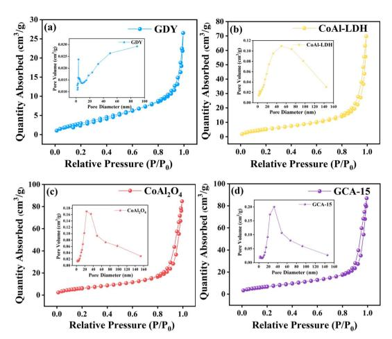
Fig. 6  $N_2$  adsorption—desorption isotherms of (a) GDY, (b) CoAl-LDH, (c) CoAl<sub>2</sub>O<sub>4</sub> and (d) GCA-15 samples (inset images are the corresponding pore size distribution curves).
