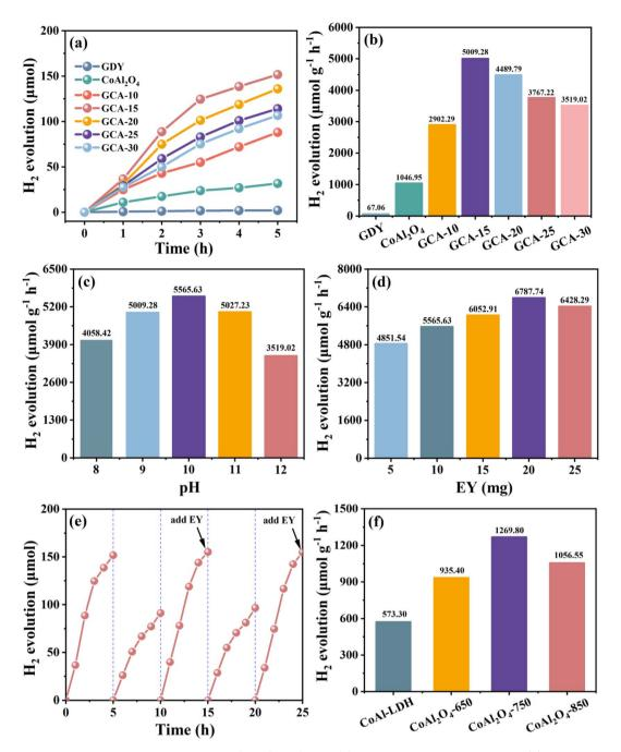
Fig. 7 (a) Photocatalytic hydrogen evolution activities of GDY,  $CoAl_2O_4$  and GCA-X under visible light irradiation; (b)  $H_2$  evolution rates of GDY, CoAl<sub>2</sub>O<sub>4</sub> and GCA-X; photocatalytic H<sub>2</sub> evolution at different (c) pH and (d) EY values for GCA-15; (e) photostability of the GCA-15 photocatalyst; (f) H<sub>2</sub> evolution of CoAl-LDHs, CoAl<sub>2</sub>O<sub>4</sub>-650, CoAl<sub>2</sub>O<sub>4</sub>-750 and CoAl<sub>2</sub>O<sub>4</sub>-850.
