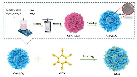
Fig. 1 Schematic of the fabrication process for CoAl<sub>2</sub>O<sub>4</sub> nanoflowers and the 2D/3D GDY/CoAl<sub>2</sub>O<sub>4</sub> heterojunction.
