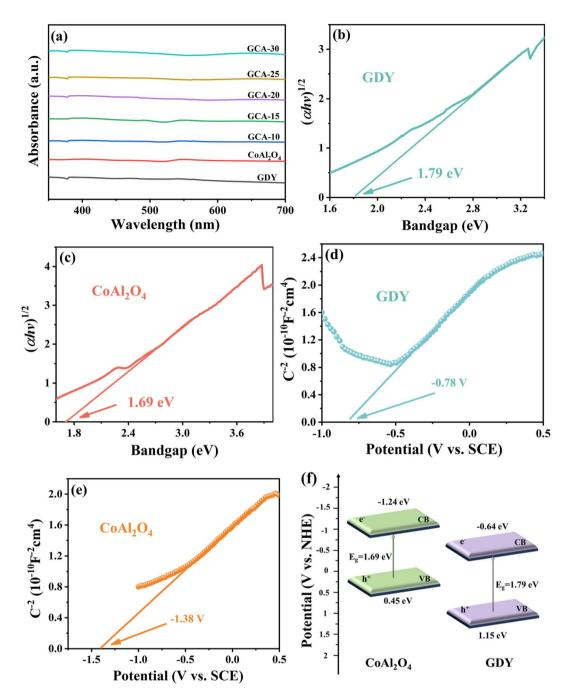
Fig. 8 (a) UV-vis diffuse reflection spectroscopy spectra of GDY,  $CoAl_2O_4$  and GCA-X; the  $(\alpha h v)^2$  vs. photo energy curves of (b) GDY and (c)  $CoAl_2O_4$ ; Mott–Schottky plots of (d) GDY and (e)  $CoAl_2O_4$ ; (f) band structures of the GDY and  $CoAl_2O_4$  samples.
