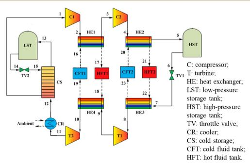
Fig. 6 A new triple production system based on transcritical Brayton cycle and carbon dioxide energy storage. 62
