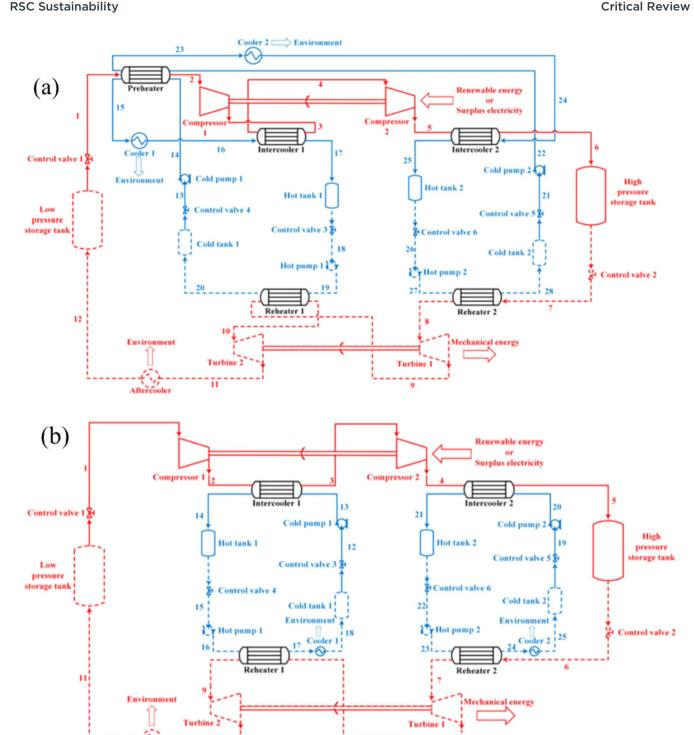
Fig. 8 (a) A cross-carbon dioxide energy storage system based on Brayton cycle;59 (b) an ultra-carbon dioxide energy storage system based on Brayton cycle.59
