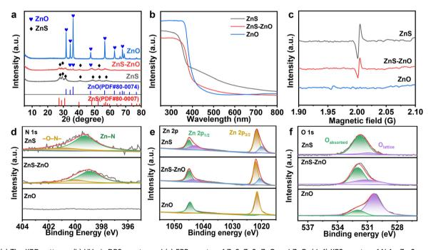
Fig. 2 (a) The XRD patterns, (b) UV-vis DRS spectra and (c) EPR spectra of ZnS, ZnS-ZnO and ZnO; (d-f) XPS spectra of N 1s, Zn 2p and O 1s of ZnS-ZnO.
