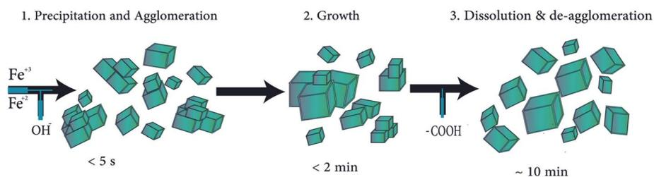
**Fig. 2** Suggested particle mechanism during the co-precipitation procedure: (1) particles are precipitated and agglomerated within 5 s, (2) agglomerated pieces grow over the next 2 or 3 min and (3) addition of neutralization solution causes particles to de-agglomerate within 10 min.
