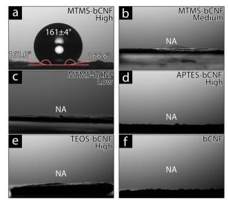
Fig. 5 Water contact angle of pressed aerogel materials.
