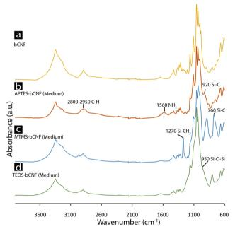
Fig. 3 FTIR spectra of the freeze-dried samples. bCNF (a), APTES-bCNF (Medium) (b), MTMS-bCNF (Medium) (c), and TEOS-bCNF (Medium) (d)
