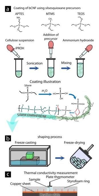
Fig. 1 Illustration of the methodology for producing silsesquioxanebCNF aerogel and methodology for thermal conductivity measurements. Coating reaction of bCNF via the addition of silsesquioxane precursors (a).31,32 Aerogel shaping and drying procedure utilizing freeze casting and freeze-drying (b). Determination of thermal conductivity of aerogel materials (c)
