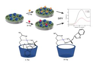
Fig. 7 Schematic representation the of electrochemical chiral recognition of tryptophan isomers (reprinted from ref. 81 with permission from Elsevier).
