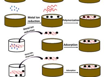
Fig. 3 Schematic representation of the different pathways used for electrode modification with metal-polymer NCs.
