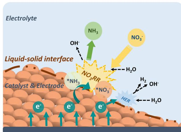
Fig. 2 The schematic illustrating the NO<sub>3</sub>RR principle on an electrode-scale.
