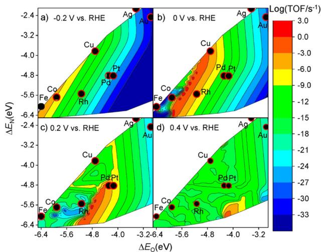
**Fig. 5** Theoretical volcano plots of the TOF as a function of atomic oxygen ( $\Delta E_{\text{O}}$ ) and nitrogen ( $\Delta E_{\text{N}}$ ) adsorption energies for electrocatalytic nitrate reduction on transition metal surfaces based on DFT-based microkinetic simulations at (a)  $-0.2$  V, (b)  $0$  V, (c)  $0.2$  V, and (d)  $0.4$  V vs. RHE by Liu *et al.* Reprinted with permission from ref. 52. Copyright 2019, American Chemical Society.
