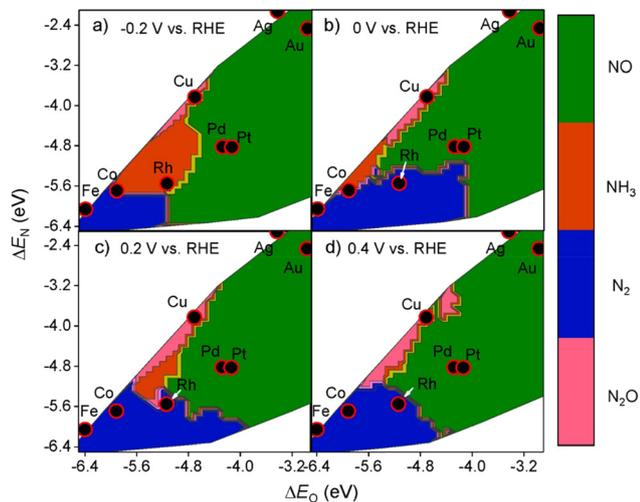
**Fig. 6** Theoretical selectivity maps to NO, N<sub>2</sub>O, N<sub>2</sub>, or NH<sub>3</sub> products from electrocatalytic nitrate reduction as a function of oxygen and nitrogen adsorption energy at (a)  $-0.2$  V, (b)  $0$  V, (c)  $0.2$  V, and (d)  $0.4$  V vs. RHE by Liu *et al.* Reprinted with permission from ref. 52. Copyright 2019, American Chemical Society.
