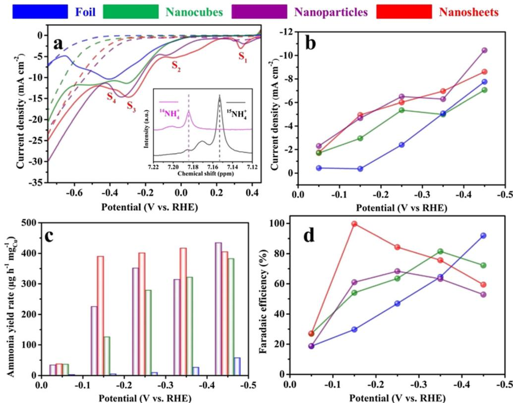
**Fig. 8** Electroreduction of nitrate to ammonia on the copper catalyst. (a) Linear sweep voltammetry curves of copper catalysts on carbon paper measured in 0.1 M KOH (dotted line) in the presence of 10 mM KNO<sub>3</sub> (solid line). Scan rate: 20 mV s<sup>-1</sup>. (b) Current densities, (c) ammonia yield rates and (d) Faradaic efficiencies of various Cu catalysts for ammonia production at different applied potentials. Preprinted with permission from ref. 76. Copyright 2020 Elsevier Ltd.
