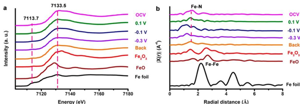
Fig. 17 (a) Fe K-edge XANES and (b) EXAFS profiles of Fe foil, FeO, Fe<sub>2</sub>O<sub>3</sub>, and FePc-pz on carbon paper under different applied potentials (from OCP, +0.1, –0.1, and –0.3 V vs. RHE, then back to OCP) by Zhong *et al.* Reprinted with permission from ref. 166 Copyright 2021 American Chemical Society.
