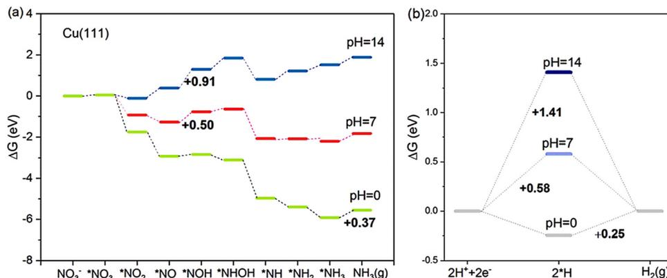
Fig. 4 The competition between (a) NO<sub>3</sub>RR and (b) HER on Cu (111) at pH = 0, 7 and 14, studied by Hu *et al.* Reprinted with permission from ref. 33. Copyright 2021, American Chemical Society.
