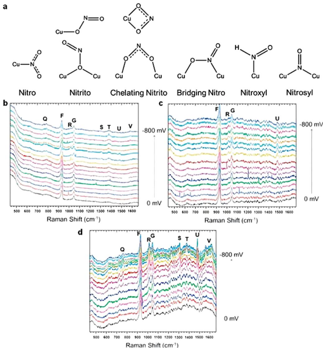
Fig. 15 (a) Adsorption modes of nitrite, nitric oxide, and HNO on the Cu surface. Electrochemical *in situ* SHINERS spectra collected from (b) Cu (100), (c) Cu (111), and (d) Cu (110) in a 0.1 M HClO<sub>4</sub> solution with 0.05 M HNO<sub>3</sub> and 10 mM HCl at a potential between 0 and -0.8 V vs. Ag/AgCl. Reprinted with permission from ref. 157 Copyright 2016 Elsevier Ltd.
