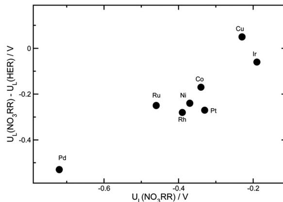
**Fig. 7** The differences between the limiting potentials for the NO<sub>3</sub>RR and HER by Xu *et al.* Reprinted with permission from ref. 26. Copyright Royal Society of Chemistry.
