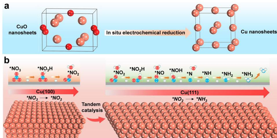
Fig. 9 Schematic illustration for enhancing the electrochemical  $NO_3RR$  over Cu nanosheets via tandem catalysis. (a) Electrochemical *in situ* reduction of the as-prepared CuO nanosheets during  $NO_3RR$ . (b) Tandem interaction of Cu (100) and Cu (111) facets. Reprinted with permission from ref. 100. Copyright 2023 Wiley-VCH Verlag GmbH.
