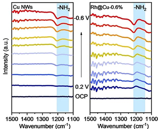
Fig. 13 Electrochemical *in situ* infrared spectroscopy (IR) of Rh@Cu-0.6% and Cu NWs under different potentials in a 0.1 M  $\text{Na}_2\text{SO}_4$  electrolyte (pH 11.5) with 0.1 M  $\text{KNO}_3$  by Liu *et al.* Reprinted with permission from ref. 83 Copyright 2022 Wiley-VCH GmbH.
