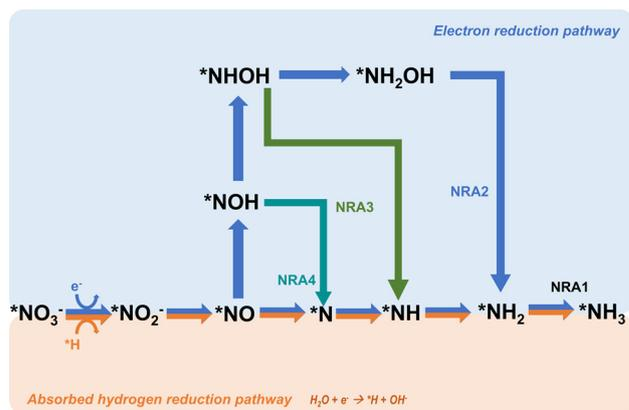
Fig. 3 The proposed direct electrocatalytic reduction pathways for nitrate reduction towards ammonia.
