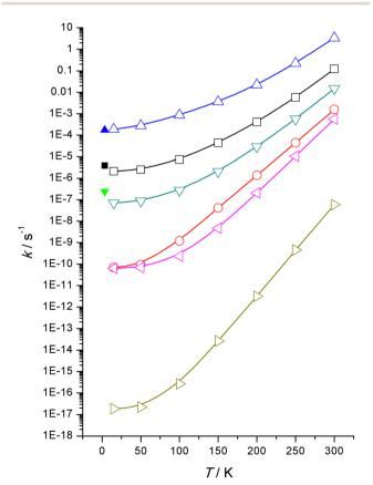
Fig. 3  $k_i/s^{-1}$  vs. T/K. MeSU3, SU3, NSU3, SU2, NNSH, 5SH. Solid symbols: experiment
