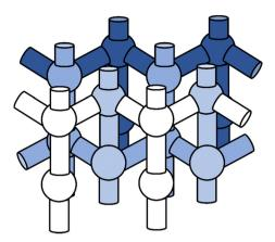
Fig. 2 Topology of the MFI framework featuring straight and zigzag channels as well as intersection regions.
