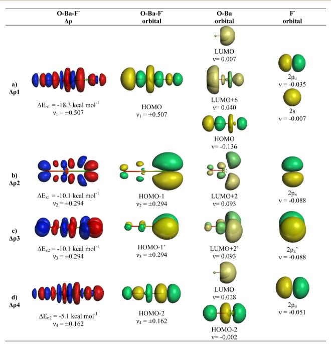
Fig. 10 Plot of deformation densities  $\Delta \rho$  of OBaF $^-$ . The pairwise orbital interactions and the associated interaction energies ( $\Delta E_{orb}$ ) between fragments OBa (S) and  $F^-$  (S) in OBa $F^-$  of the linear structure, as well as the shape of the most important interacting MOs. The direction of the charge flow is red blue. (Isovalue 0.03e a.u.<sup>-3</sup>).
