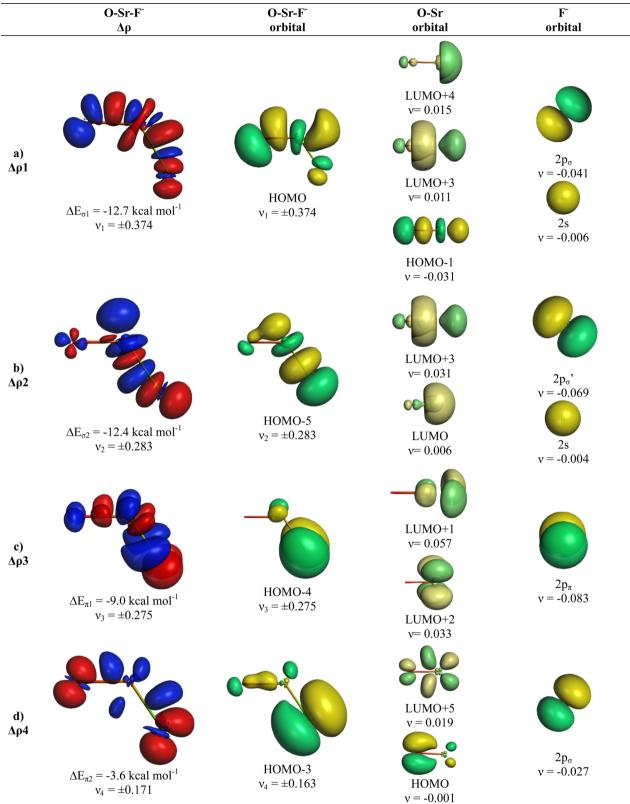
Fig. 8 Plot of deformation densities  $\Delta \rho$  of OSrF<sup>-</sup>. The pairwise orbital interactions and the associated interaction energies ( $\Delta E_{\text{orb}}$ ) between fragments OSr (S) and F<sup>-</sup> (S) in OSrF<sup>-</sup> at the equilibrium structure, as well as the shape of the most important interacting MOs. The direction of the charge flow is red  $\rightarrow$  blue. (Isovalue 0.03e a.u. $^{-3}$ ).
