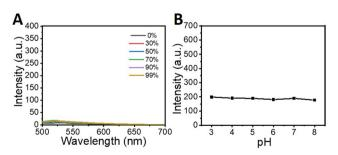
Fig. 2 In vitro tests of QMC11,  $\lambda_{ex}$ : 478 nm. (A) Fluorescence spectroscopy of QMC11 (10  $\mu$ M) in a mixture of water-ethanol with different ethanol fractions. (B) Fluorescence intensity of QMC11 (5  $\mu$ M) at different pH 3–8 (glycerin-PBS system).
