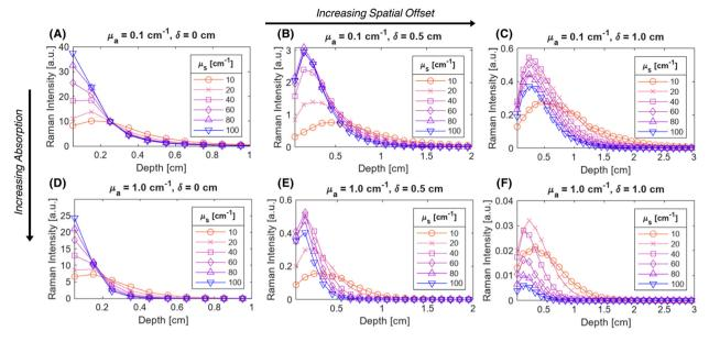
Fig. 2 Representative depth distributions of collected Raman intensity resemble left-truncated Gaussian distributions for various  $\mu_{\rm S}$ ,  $\mu_{\rm a}$ , and  $\delta$ . Depth distributions were obtained by integrating  $\eta$  over 1 mm thick layers, and are shown for  $\mu_{\rm a}$  = 0.1 cm<sup>-1</sup> (A–C) and 1.0 cm<sup>-1</sup> (D–F), and for  $\delta$  = 0 cm (A and D), 0.5 cm (B and E), and 1.0 cm (C and F).
