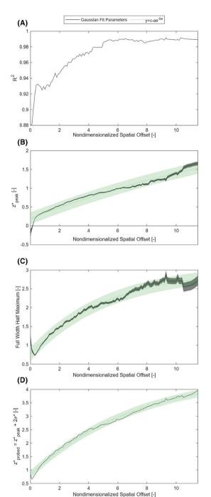
Fig. 4 Gaussian fit parameters (black) and overlaid  $y = c - ae^{-bx}$  regression curves (green); values for a, b, and c presented in Table 2. All shaded areas represent 95% confidence prediction intervals.
