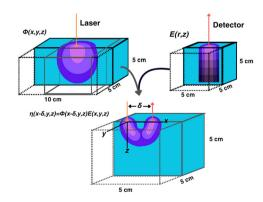
Fig. 1 Visualization of the calculation of the spatial distribution of collected Raman photon generation. Cyan represents the turbid media; purple represents magnitude of  $\phi$ , E, or  $\eta$  (brightness indicates larger
