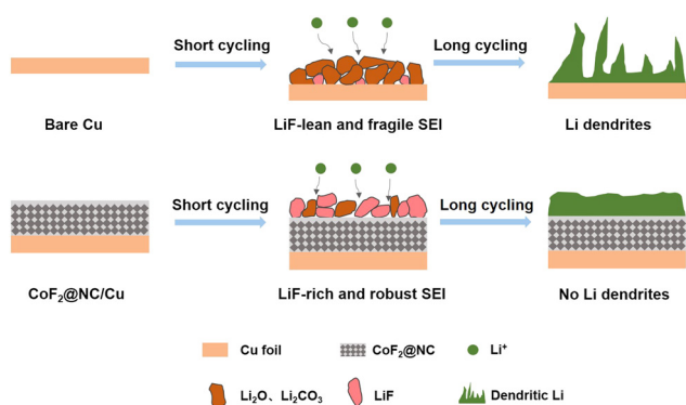
Fig. 7 Schematic illustration of the Li stripping/plating cycling on (a) bare Cu and (b) \text{CoF}_2\text{@NC/Cu} current collectors.
