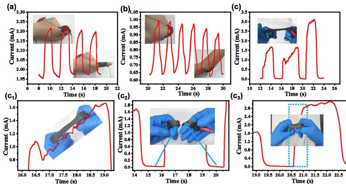
Fig. 5 Monitoring the changes of electrical signals during (a) finger and (b) elbow movements and (c–c<sub>3</sub>) material stretching under different tensile conditions based on the APC-PVA@ZnCl<sub>2</sub> sensor.
