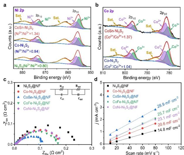
Fig. 7 XPS spectra for (a) Ni 2p and (b) Co 2p of the Ni<sub>3</sub>S<sub>2</sub>@NF, Co-Ni<sub>3</sub>S<sub>2</sub>@NF, and CoSn-Ni<sub>3</sub>S<sub>2</sub>@NF catalysts. (c) EIS analysis of Ni<sub>3</sub>S<sub>2</sub>@NF, Co-Ni<sub>3</sub>S<sub>2</sub>@NF, and CoSn-Ni<sub>3</sub>S<sub>2</sub>@NF catalysts with equivalent circuit model. (d) Linear plots of double layer charging currents with different scan rates (10–80 mV s<sup>-1</sup>) derived from CV diagrams between 0.1–0.2 V (vs. RHE).
