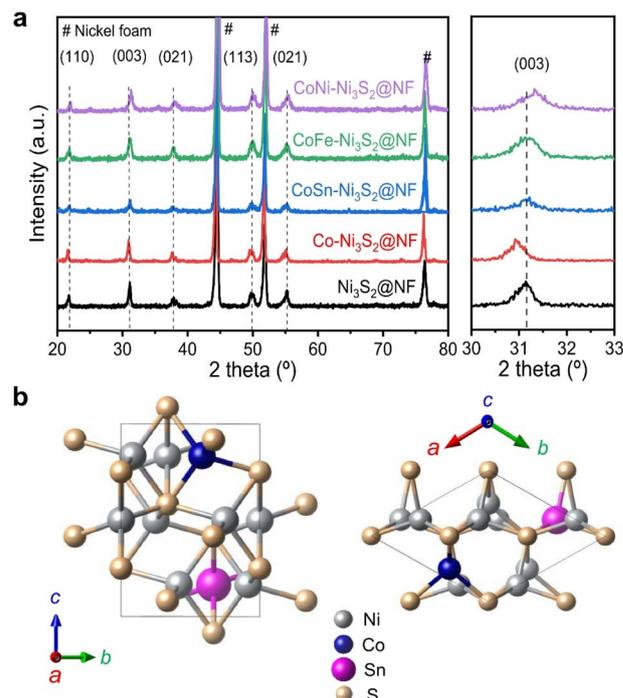
Fig. 1 Structural and phase analyses of pristine and doped- $\text{Ni}_3\text{S}_2@\text{NF}$  catalysts using XRD. (a) XRD patterns of  $\text{Ni}_3\text{S}_2@\text{NF}$  and T- $\text{Ni}_3\text{S}_2@\text{NF}$  (T = Co, CoSn, CoFe, and CoNi) catalysts. (b) Heazlewoodite structure of  $\text{CoSn-Ni}_3\text{S}_2$  phase with a space group of  $R32$  (155).
