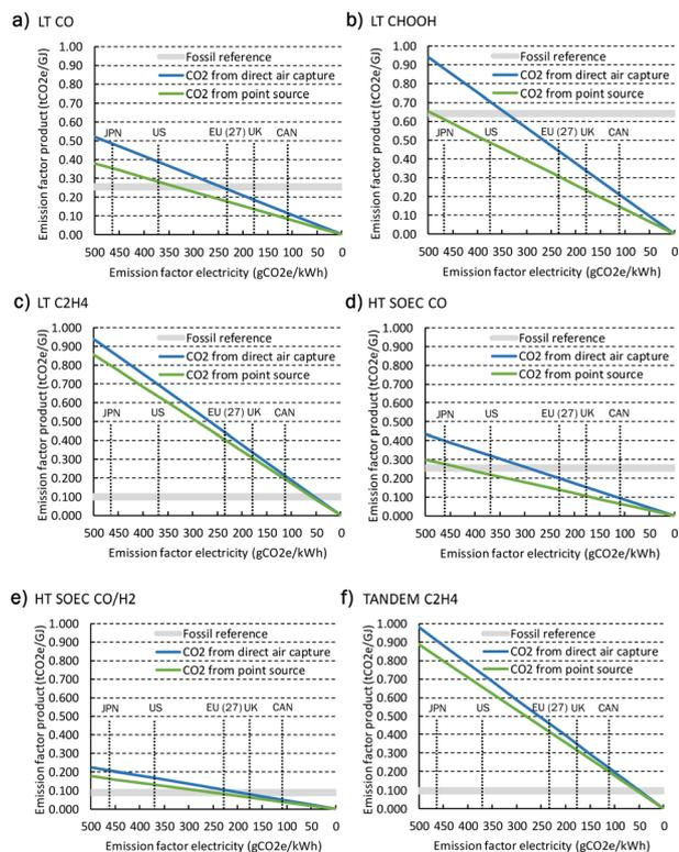
Fig. 32 Emissions from electricity use for the six electrochemical CO<sub>2</sub> conversion routes. The vertical dotted lines indicate the emission factor of the grid in a specific country/region in 2020.
