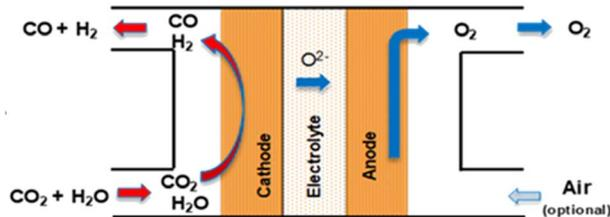
Fig. 15 Schematic concept of a SOE cell for HT co-electrolysis of steam and CO<sub>2</sub> to produce syngas.
