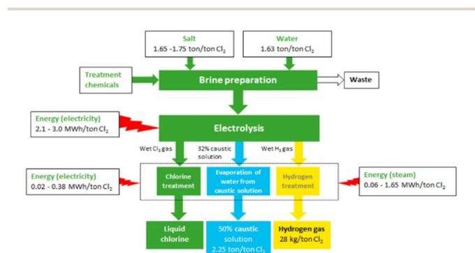
Fig. 2 Overview of the chlor-alkali production process and the main material flows (reproduced from ref. 22).
