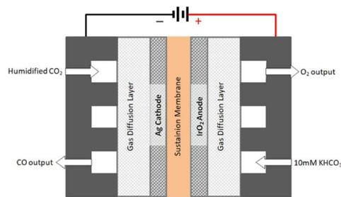
Fig. 5 Schematics of a typical membrane electrode assembly (MEA) cell for CO<sub>2</sub> electrolysis to CO (reproduced from Liu *et al.*, 2018).<sup>34</sup>
