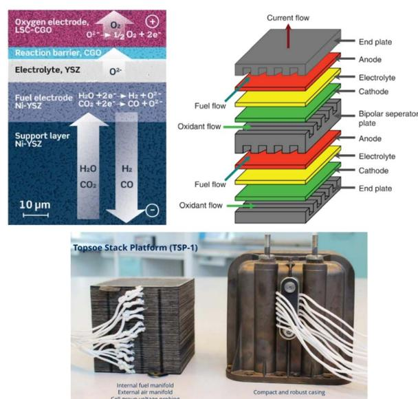
Fig. 13 Top left: electrode supported solid oxide cell design (reproduced from Hauch *et al.*, 2020).<sup>55</sup> top right: scheme of two single repeating SOC units design in a SOE stack (reproduced from Singhal, 2014).<sup>56</sup> bottom left: Topsoe stack design developed for CO production (reproduced from Küngas *et al.*, 2019).<sup>58</sup>
