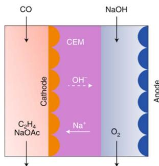
Fig. 20 CO electrolyser design for the production of  $C_2H_4$ , with a CEM and an alkaline anolyte for the OER. Reproduced from Jouny *et al.*, 2019.<sup>82</sup>
