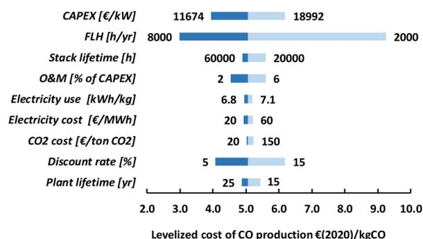
Fig. 23 Sensitivity analysis for route 1 – LT electrochemical conversion of CO<sub>2</sub> to CO. Nine parameters are varied to explore their effect on the current base-case levelized cost of CO production. The fossil reference CO price amounts to 0.07–0.18€ per kg<sub>CO</sub>.
