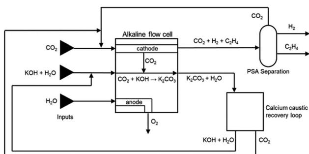
Fig. 11 Process flow diagram for CO<sub>2</sub> reduction towards ethylene in an alkaline flow cell. Reproduced from Sisler *et al.* (2021).<sup>51</sup>
