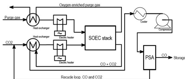
Fig. 14 Block flow diagram for Topsøe's eCOS unit for the SOE CO<sub>2</sub> to CO process (Duhn, 2017).<sup>57</sup>
