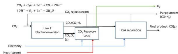
Fig. 4 Process diagram of the LT CO<sub>2</sub> electrolysis towards CO.
