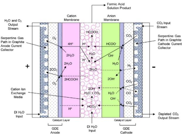
Fig. 8 Schematic representation of the 3-compartment electrochemical cell for the direct production of FA through an LT  $CO_2$  electrolysis process, showing proposed electrochemical reactions and ion transport. Reproduced from Yang *et al.*, 2017.<sup>46</sup>
