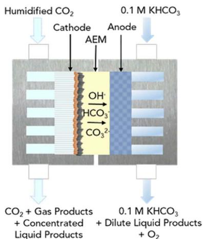
Fig. 10 Schematic diagram of the MEA cell for the LT electrolysis of CO<sub>2</sub> to C<sub>2</sub>H<sub>4</sub>. Reproduced from Gabardo *et al.* (2019).<sup>50</sup>
