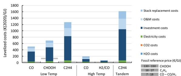
Fig. 22 Base case levelized production costs of different CO<sub>2</sub> electrochemical conversion routes. A breakdown of the costs is indicated by the coloured areas for each of the key cost components. Note the strong uncertainty related to CAPEX assessment of early stage technologies which have never been built and operated in a commercial environment. More details can be found in the enlarged diagrams in Fig. 25–30.
