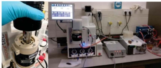
B: Alkane functionalization using decatungstate photocatalysis in continuous flow
