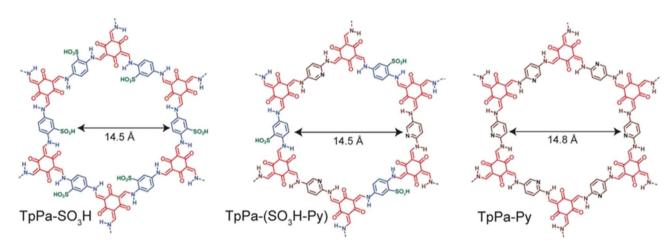
Fig. 10 Structure of TpPa-SO<sub>3</sub>H, TpPa-(SO<sub>3</sub>H-Py) and TpPa-Py. Reprinted with permission, <sup>62</sup> Copyright (2016) from American Chemical Society.
