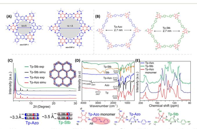
Fig. 2 (A) Chemical structure of aza-COF-1 and aza-COF-2. Reprinted with permission,<sup>49</sup> Copyright (2019) from American Chemical Society. (B) Chemical structure of Tp-Azo and Tp-Stb. (C) Simulated and experimental PXRD pattern of Tp-Azo & Tp-Stb. (D) FTIR spectra of Tp-Azo, Tp-Stb and their monomers. (E) <sup>13</sup>C NMR spectra of Tp-Azo & Tp-Stb with reference to Tp-Azo monomer (red). Reprinted with permission,<sup>50</sup> Copyright (2014) from American Chemical Society.
