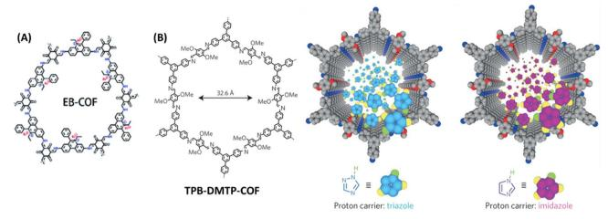
Fig. 13 (A) Structure of EB-COF. Reprinted with permission, <sup>67</sup> Copyright (2020) from Royal Society of Chemistry. (B) Structure of TPB-DMTP-COF and the graphic representation of triazole and imidazole in the channels. Reprinted with permission, 68 Copyright (2016) from Nature publications.
