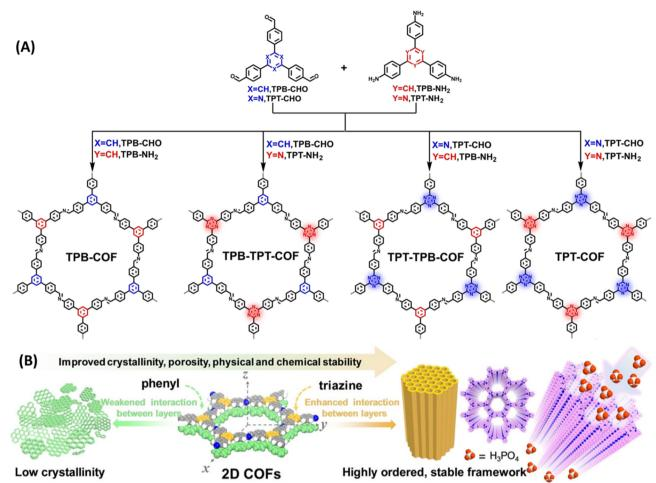
Fig. 7 (A) Bottom-up strategy for the synthesis of TPB-COF, TPB-TPT-COF, TPT-TPB-COF, and TPT-COF. (B) Schematic illustration of the crystallite growth controlled by  $\pi-\pi$  stacking interactions between layers. Reprinted with permission,<sup>57</sup> Copyright (2022) from Wiley.
