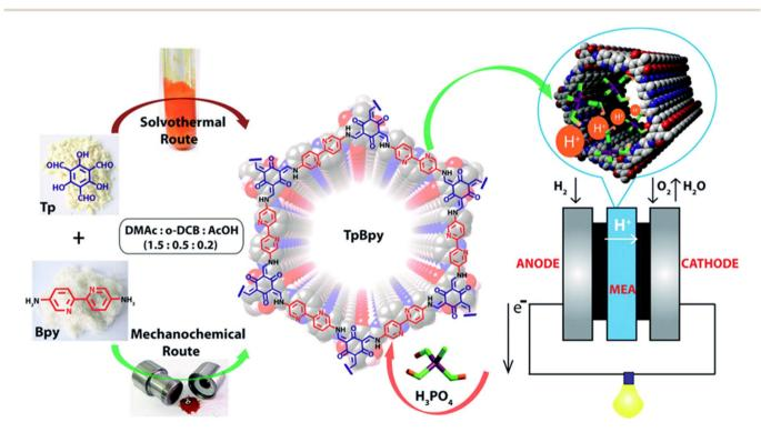
Fig. 3 Synthesis of TpBpy COF via solvothermal and mechanochemical routes, doping of  $H_3PO_4$  and their implementation in fuel cell as solid electrolyte. Reprinted with permission, <sup>51</sup> Copyright (2016) from Royal Society of Chemistry.
