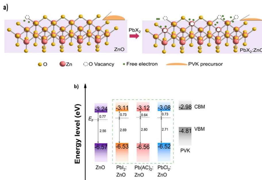
Fig. 22 (a) Energy level alignment of ETLs and the perovskite layer. (b) Visualization of the impact of the enhanced oxygen vacancy in  $PbX_2$ :ZnO. This figure has been reproduced from ref. 136 with permission from Wiley, copyright 2022.
