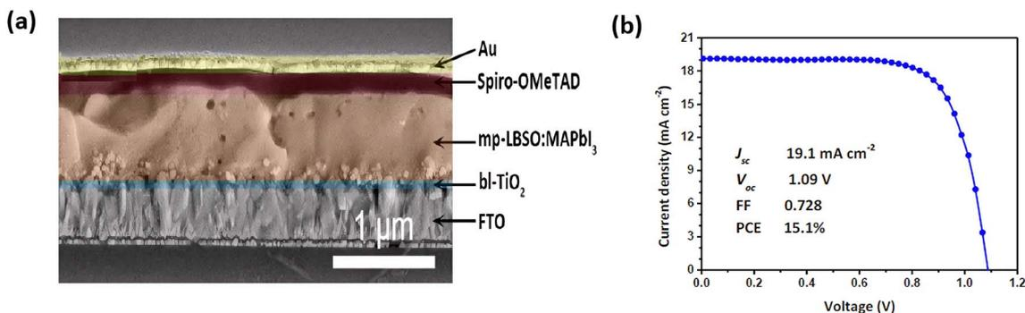
Fig. 10 (a) A cross-sectional view of SEM images from La-doped BSO in PSC. (b)  $J$ - $V$  curves of La-doped BSO in PSC under AM 1.5 illumination. Reproduced with permission from ref. 68. Copyright 2017 Royal Society of Chemistry.
