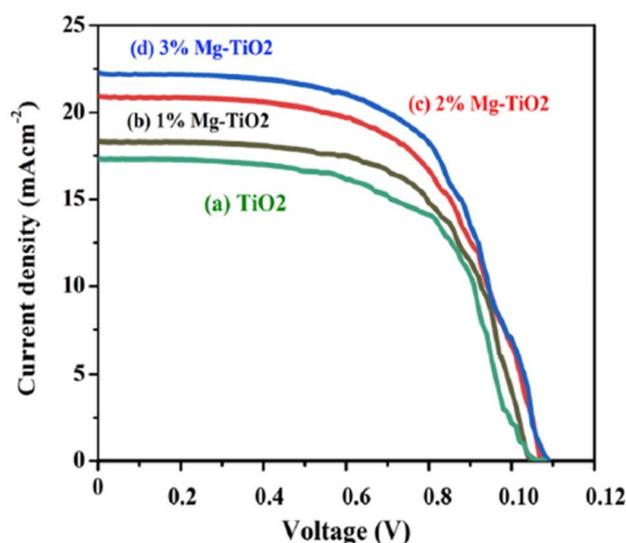
Fig. 8 J-V characteristics of PSC based on (a) bare TiO<sub>2</sub>, (b) 1% Mg-doped TiO<sub>2</sub>, (c) 2% Mg-doped TiO<sub>2</sub>, and (d) 3% Mg-doped TiO<sub>2</sub>. Reproduced with permission from ref. 49. Copyright 2021 Elsevier.
