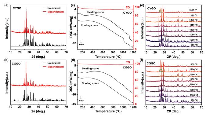
Fig. 1 (a and b) Experimental and theoretical PXRD patterns of CYGO and CGGO: (c and d) TG-DSC curves of CYGO and CGGO: (e and f) the PXRD patterns evolution of CYGO and CGGO polycrystalline pure phases under elevated temperature conditions.
