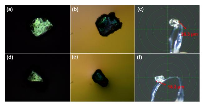
Fig. 5 (a-c) The original interference color, extinction and thickness of the CYGO crystal, respectively; (d-f) the original interference color, extinction and thickness of the CGGO crystal, respectively.
