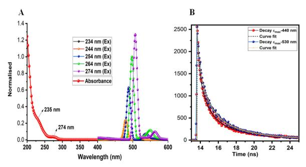
Fig. 3 (A) UV-Vis spectra of YGQDs (red) and PL spectra of YGQDs recorded at different excitation wavelengths (234 nm  $\rightarrow$  274 nm). (B) Picture representing the ns lifetime decay of YGQDs at 440 nm (red) and 530 nm (blue), respectively.
