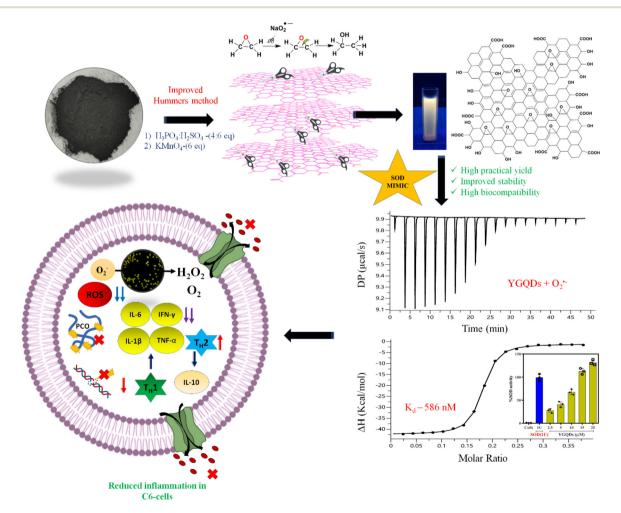
Scheme 1 Schematic illustrations of YGQDs synthesis, characterization, O2. with Kd values, and antioxidant effect with selective SOD-like activity against oxidatively-stressed C6-cell survival indicating the roles of pro-inflammatory and anti-inflammatory cytokines release.
