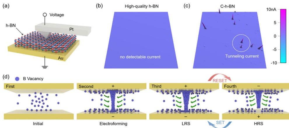
**Fig. 4** Physical mechanism of the C-h-BN-based memristors. (a) Schematic diagram of the conductive atomic force microscope (C-AFM) experiments. (b) Current mapping image of the Pt/h-BN/Au cell with high-quality h-BN flakes. (c) Current mapping image of the Pt/C-h-BN/Au cell with the as-prepared C-h-BN flake. (d) Schematic diagram of the resistive switching process. It includes the initial state, electroforming process, LRS after the SET process and HRS after the RESET process, respectively.
