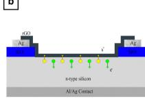
Fig. 2 (a) Schematic of a graphene-on-semiconductor (Si) solar cell. (b) Electron-hole pairs transport across the surface junction. Reproduced from ref. 159, with permission from Elsevier.
