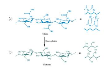
Fig. 15 Chemical structure and possible intermolecular hydrogen bonding (--) in (a) chitin and (b) chitosan.
