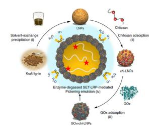
Fig. 12 Preparation of GOx-chi-LNPs and application in enzymedegassed SET-LRP-mediated Pickering emulsion (Schematic). (i) Preparation of LNPs via solvent-exchange precipitation. (ii) Adsorption of chitosan on LNPs to yield chi-LNPs. (iii) Adsorption of GOx on chi-LNPs to yield Gox-chi-LNPs. (iv) Application of GOx-chi-LNPs as biocatalytic degassing stabilizers for SET-LRP in Pickering emulsion media. Reproduced from ref. 92 with permission from Nature Portfolio, copyright 2020.
