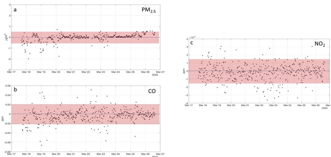
Fig. 4 Ten-day co-location data showing the difference between values measured in tube 2 minus tube 1. The expected difference for co-location would equal 0. Red shaded area denotes the  $\pm$  uncertainty assigned to each measurement. >90% of the data are included within the shaded area. (a) PM<sub>2.5</sub>  $\pm$  0.5  $\mu\text{g m}^{-3}$ . (b) CO  $\pm$  0.02 ppm (c) NO<sub>2</sub>  $\pm$  0.0015 ppm.
