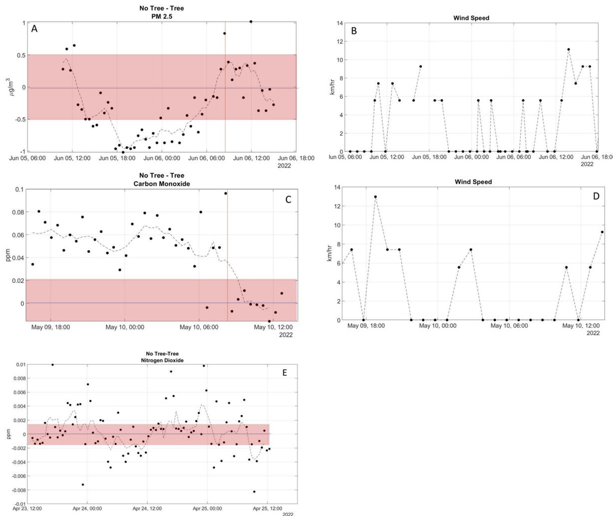
Fig. 6 (A) Difference between  $\text{PM}_{2.5}$  in ambient air (tube 2) and tree canopy air (tube 1) vs. time. Tubes are co-located following the time indicated by the vertical red line. Dashed line is a 4-point running average. (B) Wind speed during the  $\text{PM}_{2.5}$  experiment (C) same as (A) but for CO. (D) Wind speed during the CO experiment. (E) The difference between  $\text{NO}_2$  in ambient and tree canopy air. Dashed line is a 4-point running average.
