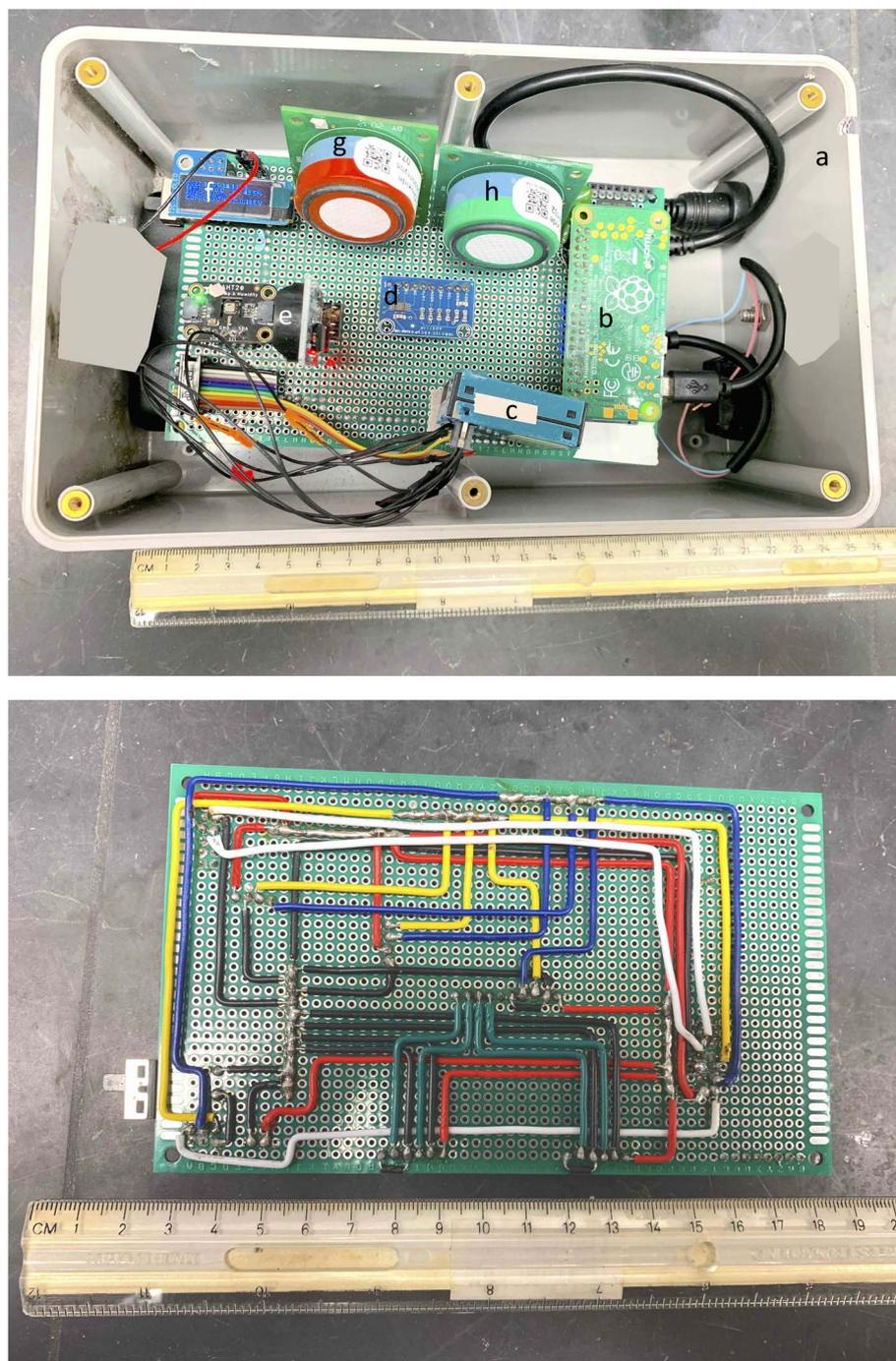
Fig. 2 (A) Photograph of sensor circuit board with components (a) plastic box, (b) Raspberry Pi computer, (c) PM<sub>2.5</sub> sensor, (d) A/D converter, (e) temperature and humidity recorder, (f) LED, (g) NO<sub>2</sub> sensor, (h) CO sensor. (B) Back of circuit board with wiring.
