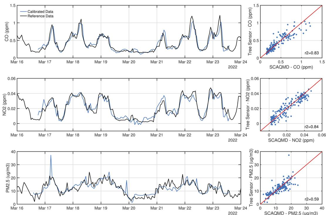
**Fig. 3** Time series and direct comparison of the tree sensor data (blue line) and the SCAQMD reference data (black line). The tree sensor data shown here is optimized to a best fit to the SCAQMD data. The red lines in the plots on the right indicate the 1 : 1 line between these two data. *R*-Squared values are 0.83, 0.84, and 0.59 for CO, NO<sub>2</sub> and PM<sub>2.5</sub>, respectively.
