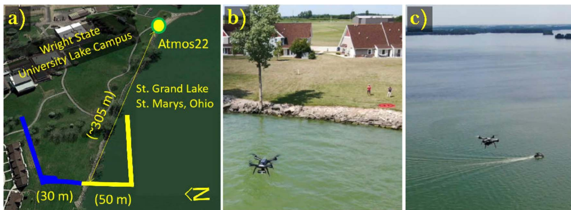
Fig. 1 (a) A schematic of the multirotor sUAS operations performed on August 5th and 6th, 2019 to measure wind variability across onshore and offshore sampling locations at Grand Lake St. Marys, Ohio. (b) An image of the multirotor sUAS hovering flight operations conducted to measure wind velocity at 10 m AGL. (c) An image of multirotor sUAS steady ascending flight operations performed to measure wind velocity from 10 m to 100 m AGL.
