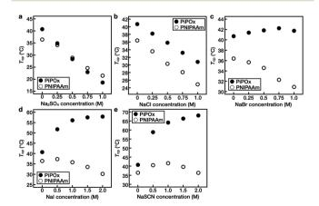
Fig. 4  $T_{\rm cp}$  profiles of PNIPAAm (open circles) and PiPOx (closed circles) in salt solutions as a function of the (a) Na<sub>2</sub>SO<sub>4</sub>, (b) NaCl, (c) NaBr, (d) NaI, and (e) NaSCN concentrations. The concentration of the polymer was 1 wt%.
