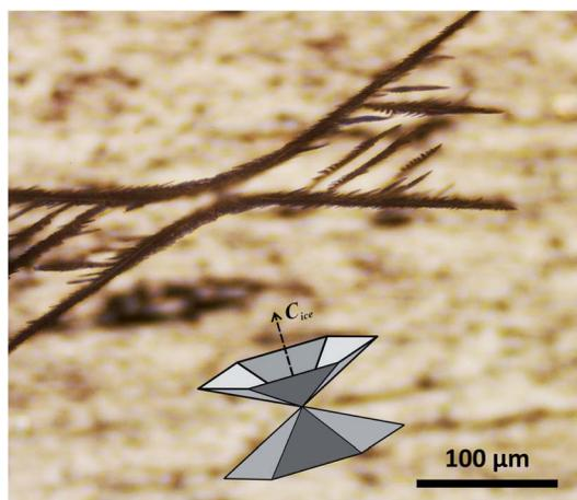
Fig. 2 3D-dendrite structure of an ice crystal in equilibrium with sucrose solution at  $-14.2$  °C. The overlay shows the structure of the inverse double pyramid of ice redrawn after Knight and DeVries,<sup>29</sup> with the orientation of the *C*-axis of the hexagonal ice crystal indicated by the arrow.
