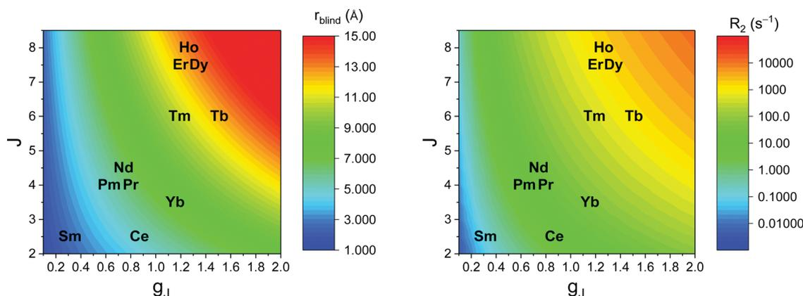
Fig. 4 Typical radii of  $^1\text{H}$  blind spheres of lanthanoid(III) ions (paramagnetic linewidths  $\geq 100$  Hz, left panel), and  $^1\text{H}$   $R_2$  PRE (right panel), due to Curie relaxation, for a proton at 10 Å from the lanthanoid ion, at 900 MHz. The electron relaxation times  $\tau_e$  are set to 1 ps and  $\tau_r$  to 10 ns. Gadolinium(III), with  $\tau_e$  several orders of magnitude larger, is shown in Fig. 3.
