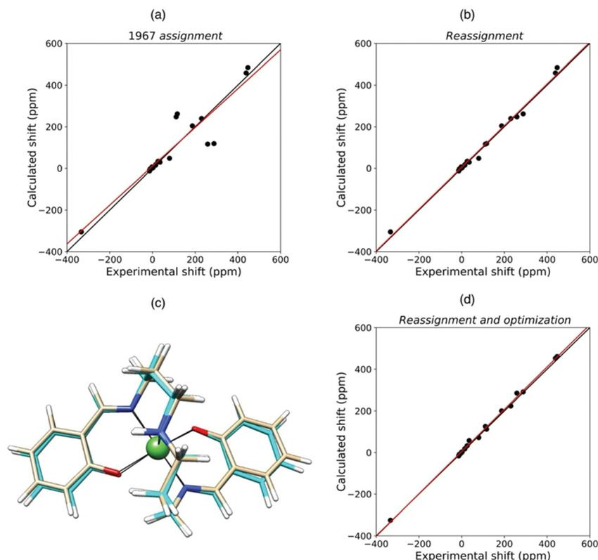
Fig. 9 Agreement between experimental and QC calculated shifts of NiSAL-HDPT, with the assignment previously reported (a),<sup>124</sup> and the theory-based reassignment (b). Comparison between initial (beige) and DFT-optimized (cyan) structures (c) and agreement between the experimental and QC calculated shifts for the refined structure (d).
